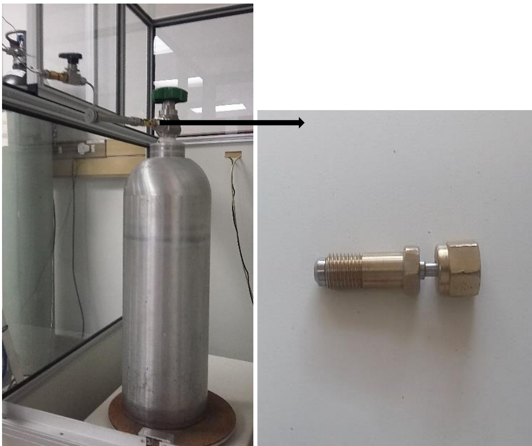
Figure 3.3: Injection system and minimum dead volume for transferring liquid sample to the cylinder
