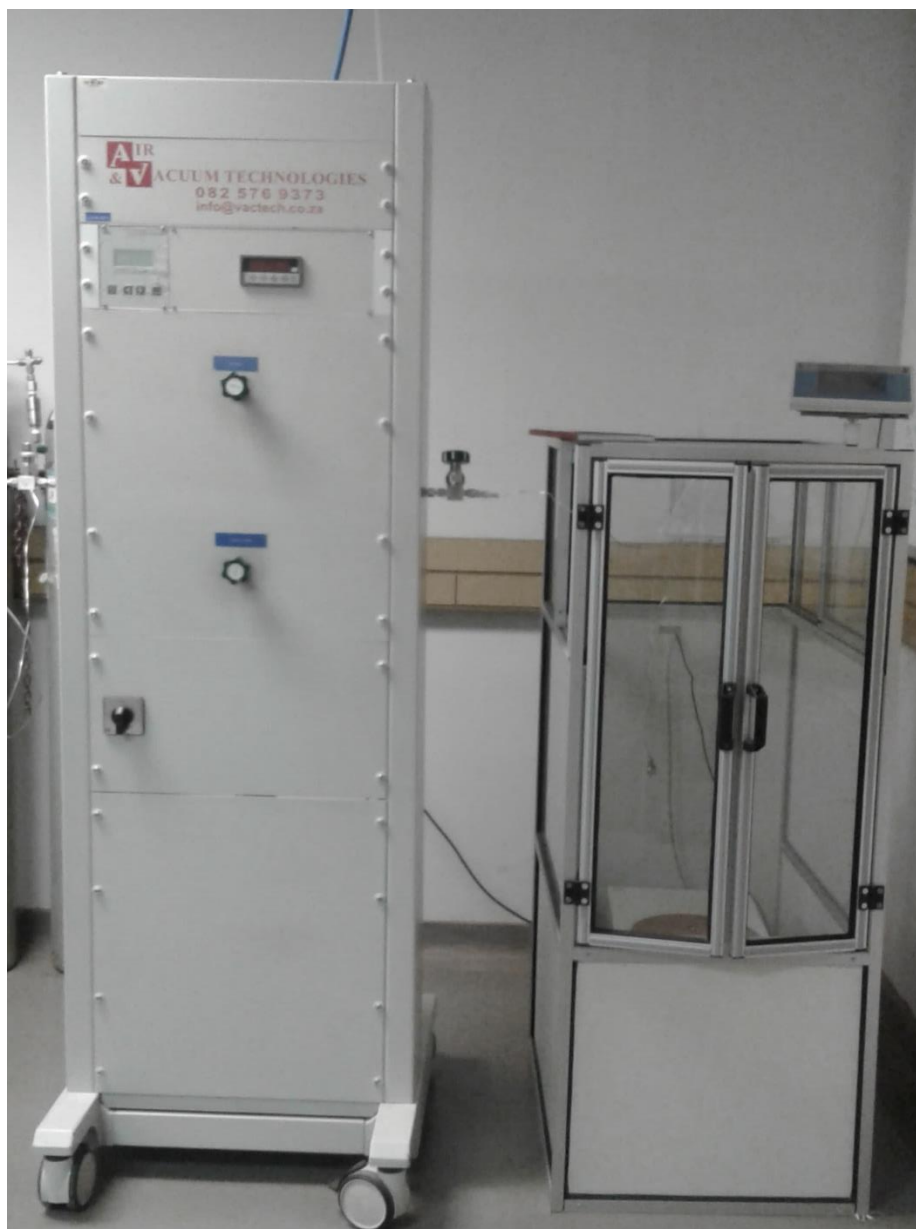
Figure 3.2: Filling system and weighing balance for transferring gas in the cylinder
