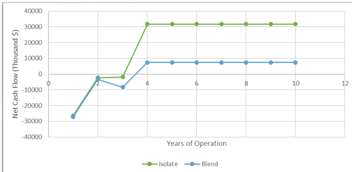
Figure 26: Net cash flow comparison of the production of CBD isolates and CBD full spectrum blends.
