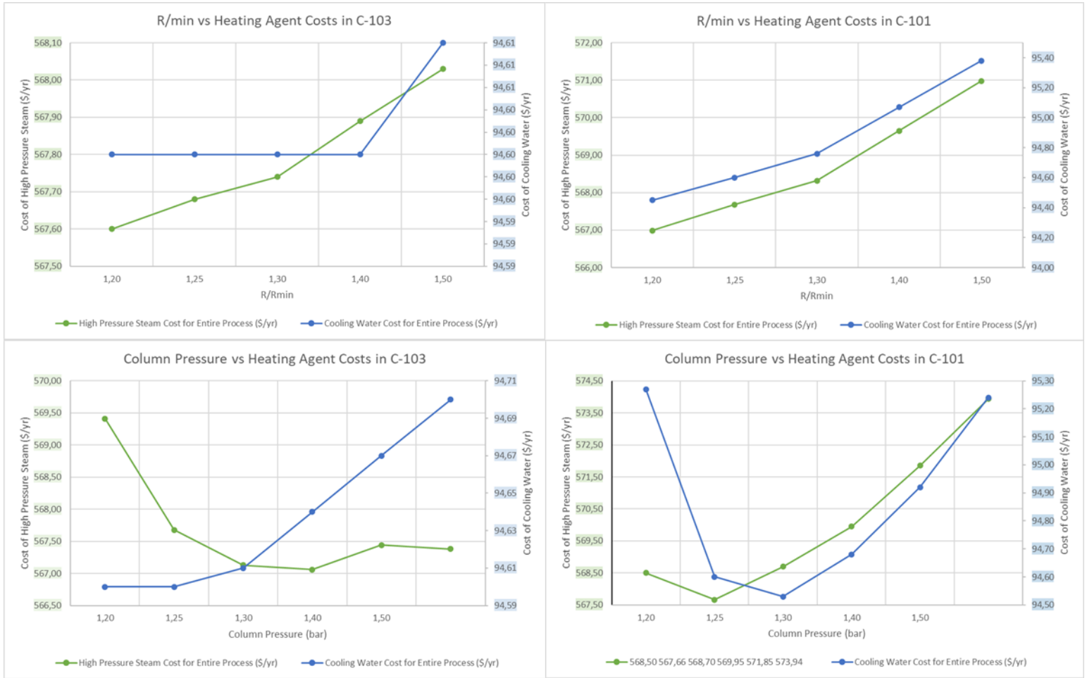
Figure 38: Additional sensitivity analysis graphs on distillation columns C-103 and C-101.
