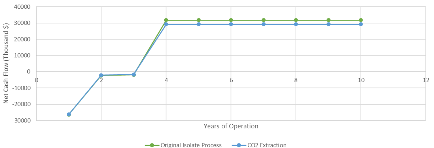
Figure 32: Net cash flow comparison of the production of CBD isolates using the original cold ethanol extraction process versus the supercritical CO 2 process.
