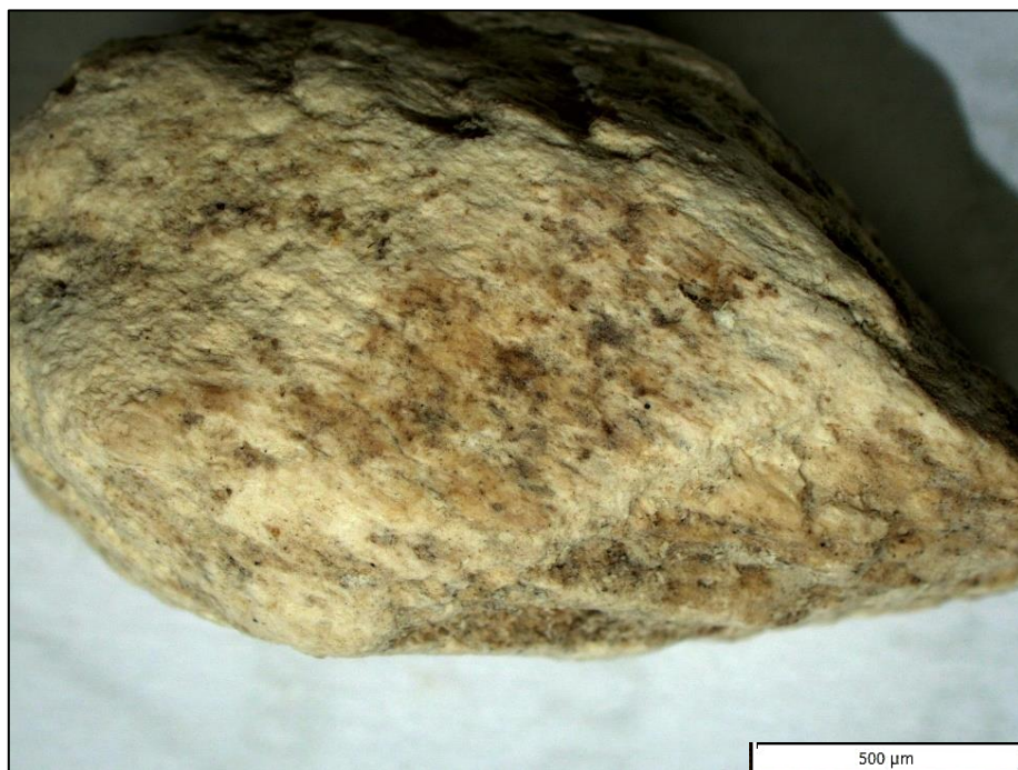
Figure B.2: Gastric acid etching on MSA III specimen
