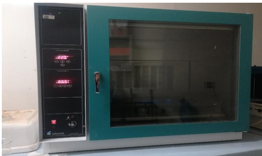
Figure 3.4: Adsorption shaking test equipment (Labcon shaking incubator)
