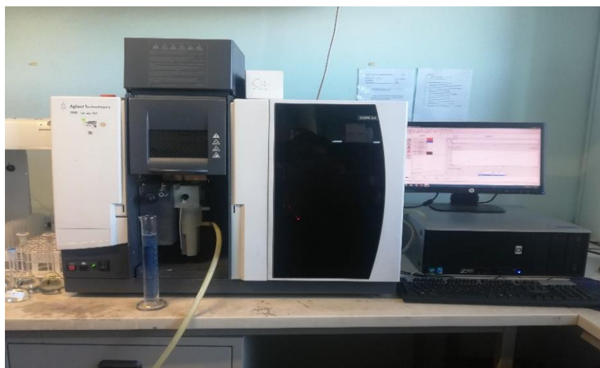
Figure 3.5: Atomic Absorption Spectrophotometer (AAS) equipment for metal ion concentration analysis
