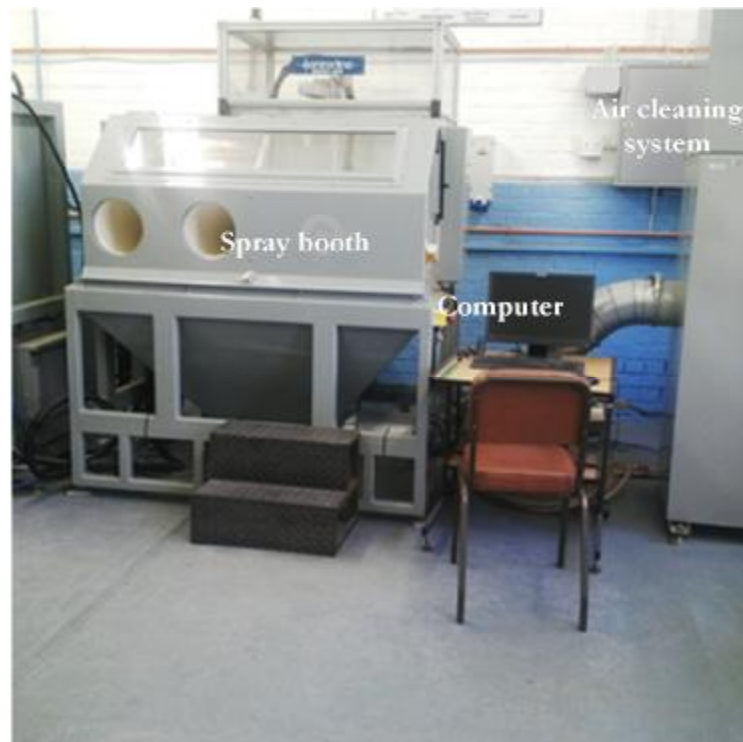
Figure 3.5. Spray booth and exhaust system (air cleaning system).
