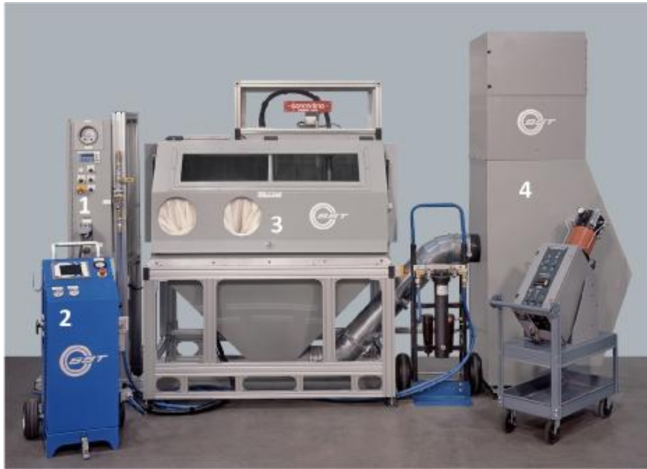
Figure 3.2. SST low-pressure cold spray system.
