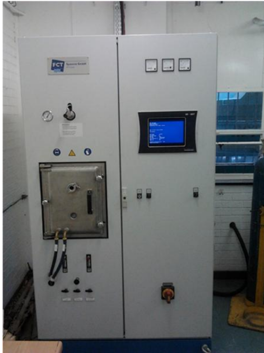
Figure 3.1. FCT HP-D5 spark plasma sintering furnace.
