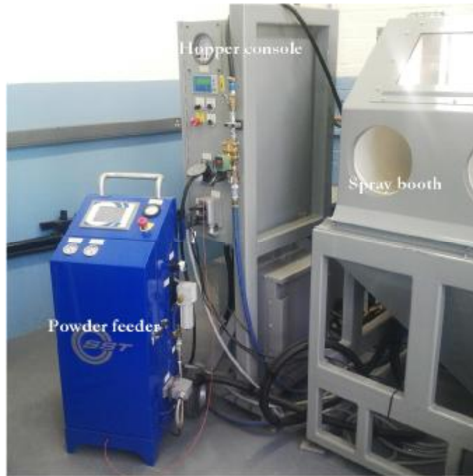
Figure 3.4. Powder feeder, hopper console and spray booth.
