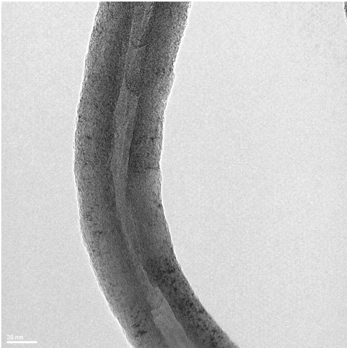
Figure 4.3: HMTEM image of CNT produced at 650°C using LaNi 5
