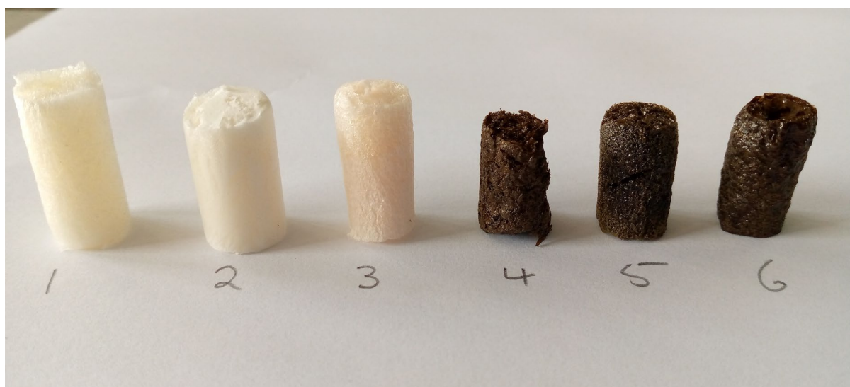
Figure 8.2: Photographed images of (1) CS, (2) Gel, (3) CS/Gel, (4) PDA/CS/Gel, (5) AgI@PDA/CS/Gel and (6) CuI@PDA/CS/Gel.
