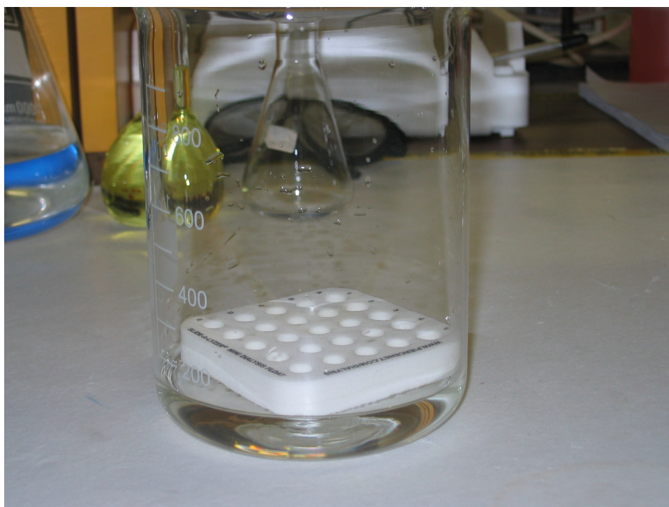
Figure 13. Photograph of minidialysis float TM immersed in dialysis buffer prior to placement in a waterbath at 37 °C for 3 hours.
