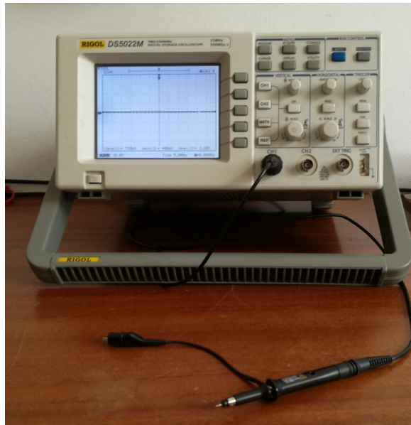
Fig. 5.9 Oscilloscope used to indirectly measure the ion beam current density.
