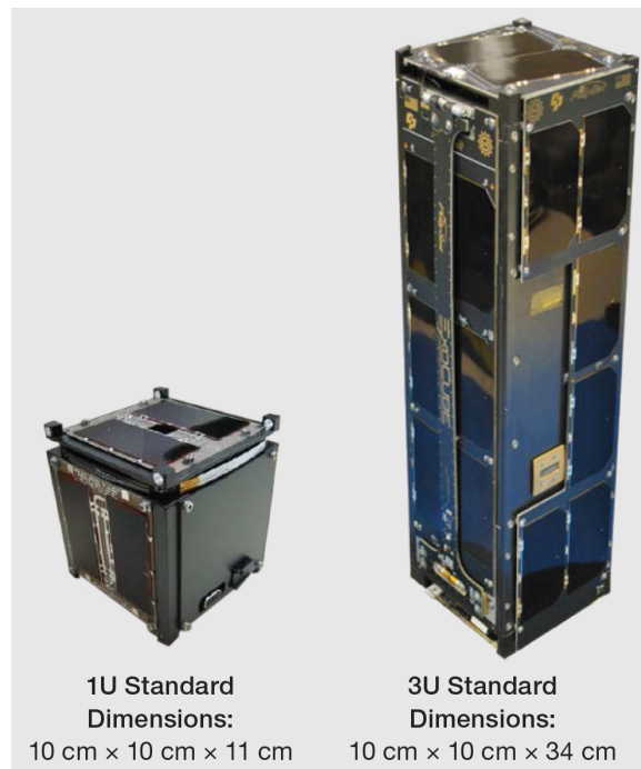
Fig. 1.1 1U and 3U CubeSat configurations developed by California Polytechnic State University [1].
