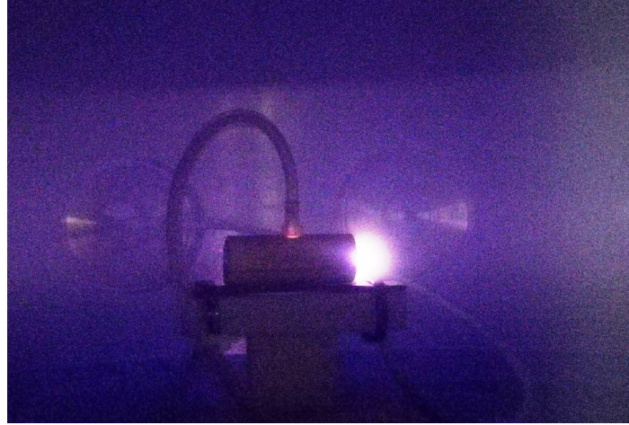
Fig. 7.13 Plume formation observed at the anode when the propellant flow rate was set above 300 ng/s. The thruster did not operate stably when the propellant flow rate was set higher than this. Despite its dramatic appearance, it is hypothesised that this plume consists predominately of electrons which do not contribute significantly to thrust.
