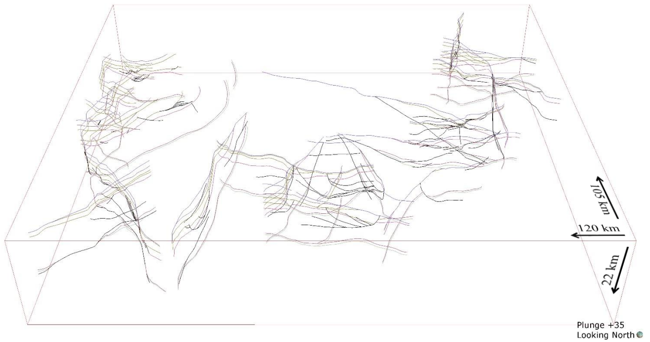
Figure 6.2.2 Digitised seismic section interpretations, including polylines of the imaged contact interfaces and fault planes.
