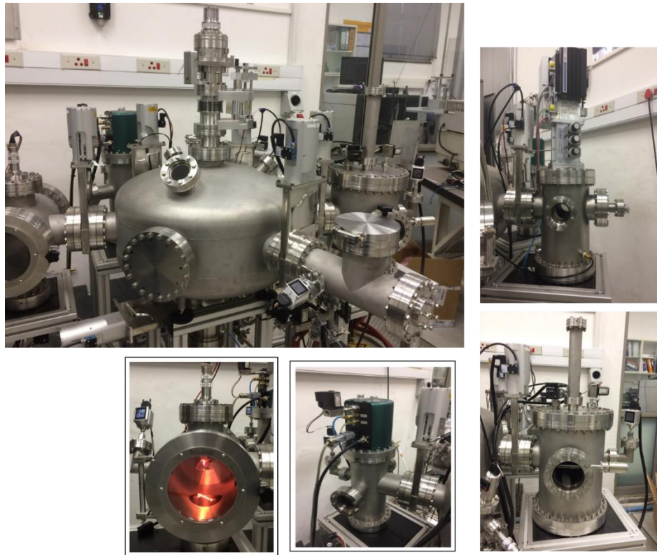
Figure 60 Multi-purpose rotating sample deposition chamber. (a) Thermal evaporation and CVD chamber. (b) RF-plasma chamber for substrate cleaning or etching. (c) Electron beam evaporating chamber with six crucible target allowing for multiple layer evaporations without breaking chamber vacuum. (d) Microwave powered CVD diamond chamber with trimethylborane gas source for the synthesis of superconducting boron doped diamond films.
