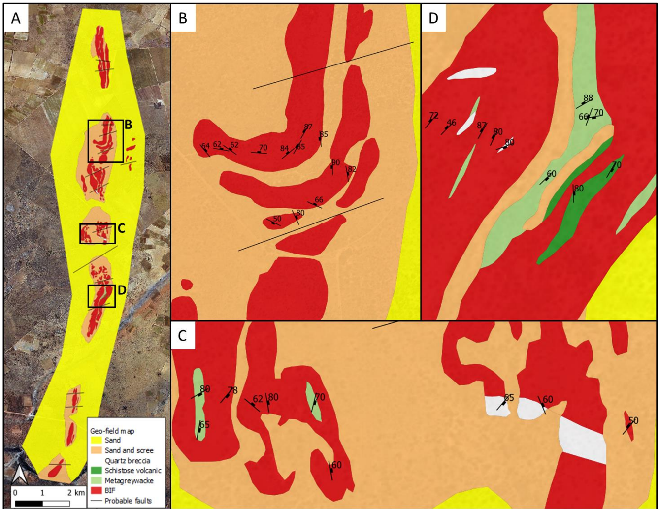
Figure 17. Geological maps of the southern part of the study area, created from field mapping and satellite imagery. (a): overview map showing various lithologies and probable faults shown in black lines. (b): synformal fold within the BIF. (c): predominantly east-dipping part of the greenstone belt. A ~20 m wide of quartz brecciation is present. (d): area with an overall antiformal structure where numerous greenstone lithologies are present.
