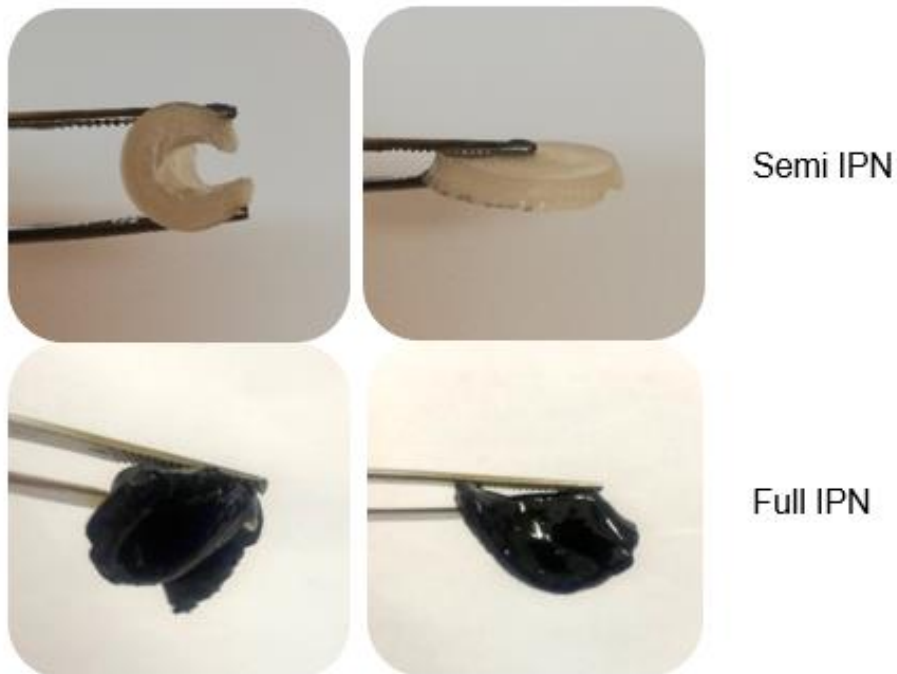
Figure 4.7: Indication of the elastic ability of the disks after 4 hours of hydration in aCSF. The semi IPN is shown at the top and the full IPN is shown at the bottom.
