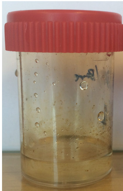
Figure A.1: Synthetic produced water after a month with an oil concentration of 1000 mg/l
