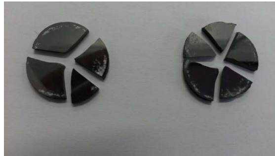
Figure 6.1 Photograph of fractured sample of 85TiC-12Al 2 O 3 -3Y 2 O 3
