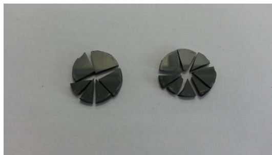
Figure 6.13 Photograph of fractured sample of 79TiC-4.5Al 2 O 3 -5.6Y 2 O 3 -4.9SiO 2 -7.1(10 vol.%) SiCw
