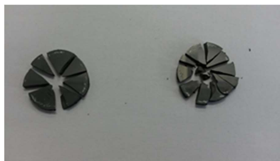
Figure 6.5 Photograph of fractured sample of 79TiC-11Al 2 O 3 -3Y 2 O 3 -7(10 vol.%) SiCw
