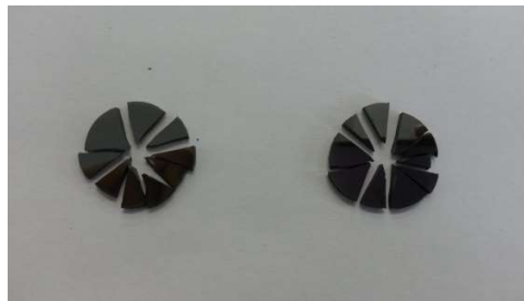
Figure 6.21 Photograph of fractured sample of 77.8TiC-6.9Al 2 O 3 -1.7Y 2 O 3 -14(20 vol.%) SiCw
