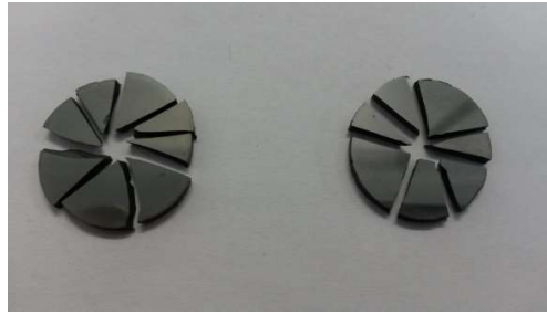
Figure 6.17 Photograph of fractured sample of 78.6TiC-3.5Al 2 O 3 -5.6Y 2 O 3 -4.9SiO 2 -7.5 (10 vol.%) cBN
