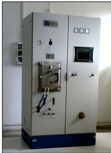
Figure 3.7 FCT group Systeme GmbH Spark Plasma Sintering Machine
