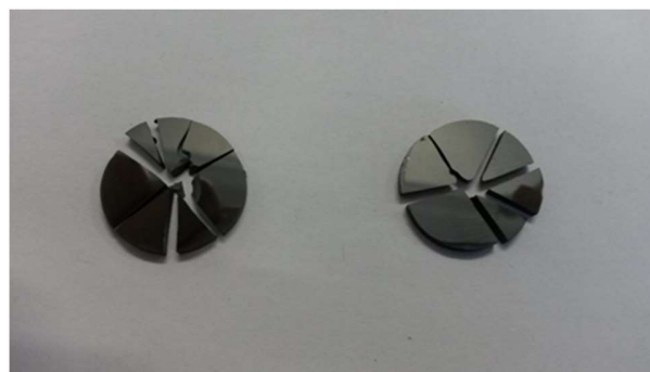
Figure 6.9 Photograph of fractured sample of 73TiC-10Al 2 O 3 -3Y 2 O 3 -14(20 vol.%) SiCw
