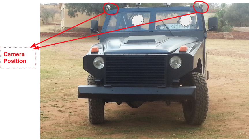
Figure 4.1 Data collection vehicle and camera mounting.
