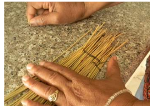
Tying the thatch together.
