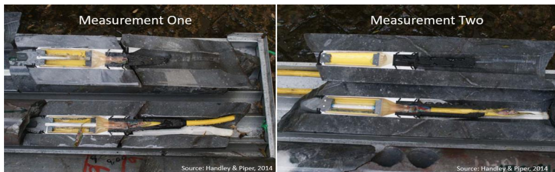
Figure 30. Sections of over core showing strain cells (Handley & Piper, 2014).
