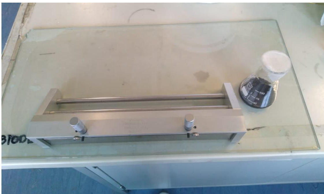
Figure 4.1. Casting blade and glass used to cast membranes.
