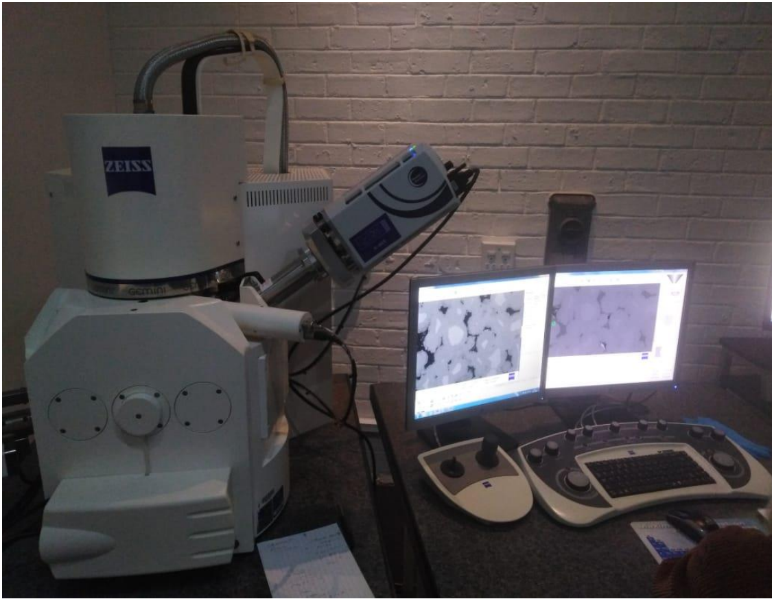
Figure 4.2. SEM (model Carl Zeiss Sigma), Germany (Wits, School of Chemical and Metallurgical Engineering).
