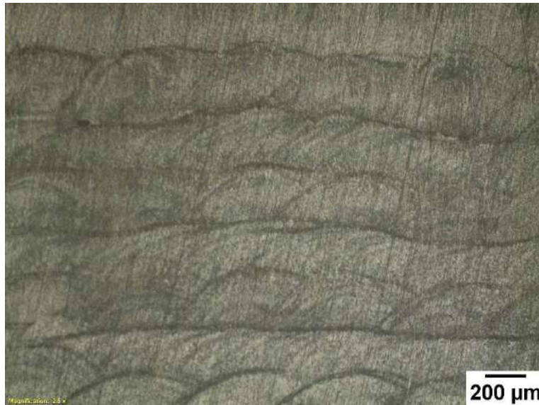
Figure 6-19: Microstructure of FeCr showing the deposition beads.
