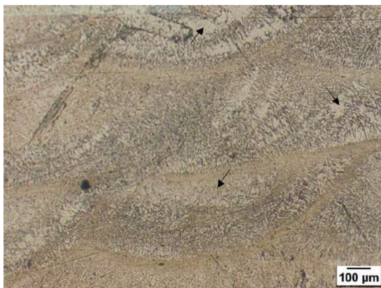
Figure 6-20: Micrograph of FeCr with arrows showing retained austenite.
