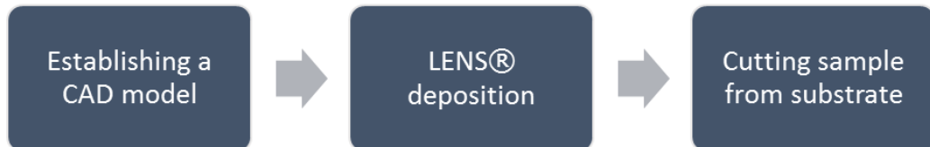
Figure 8-1: LENS® process flow for the manufacture of the prototype burr.
