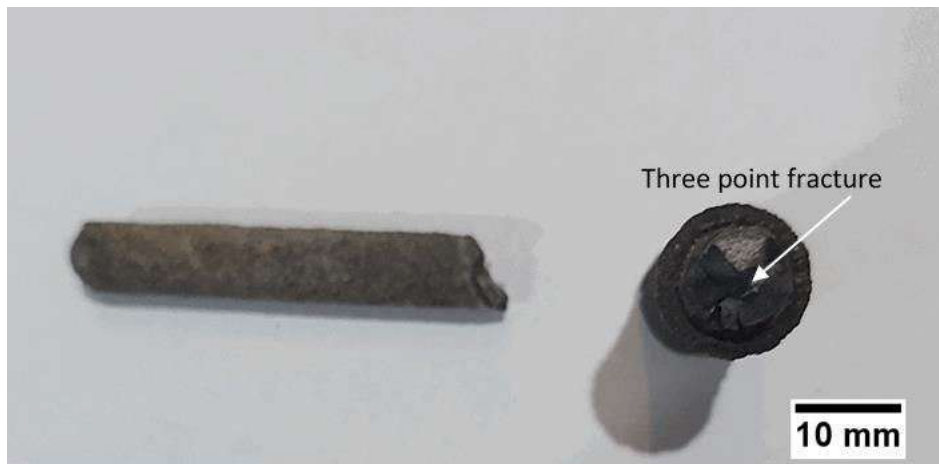
Figure 8-16: Fracture surface of LENS® fabricated rotary burr.
