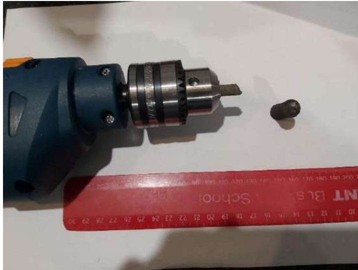
Figure 8-15: Fracture of LENS® cylindrical rotary burr.
