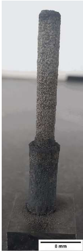
Figure 8-8: LENS® fabrication of a cylindrical rotary burr with preheat of 250°C.
