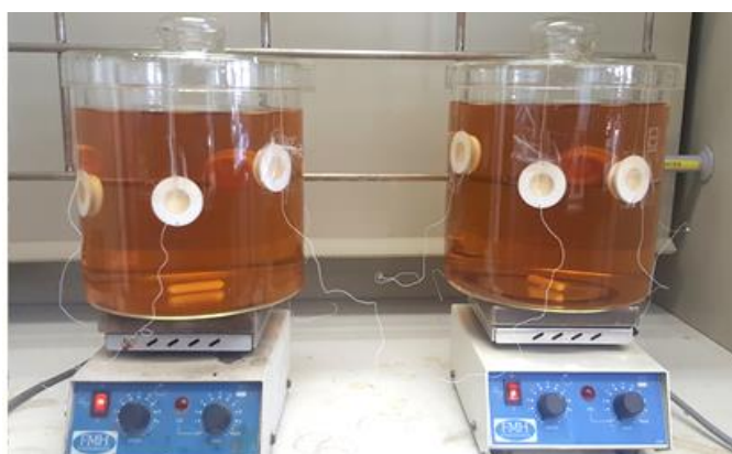
Figure 4.8: Experimental set up of SCPEI-PCPEI based DGT sampling devices in AMD water.
