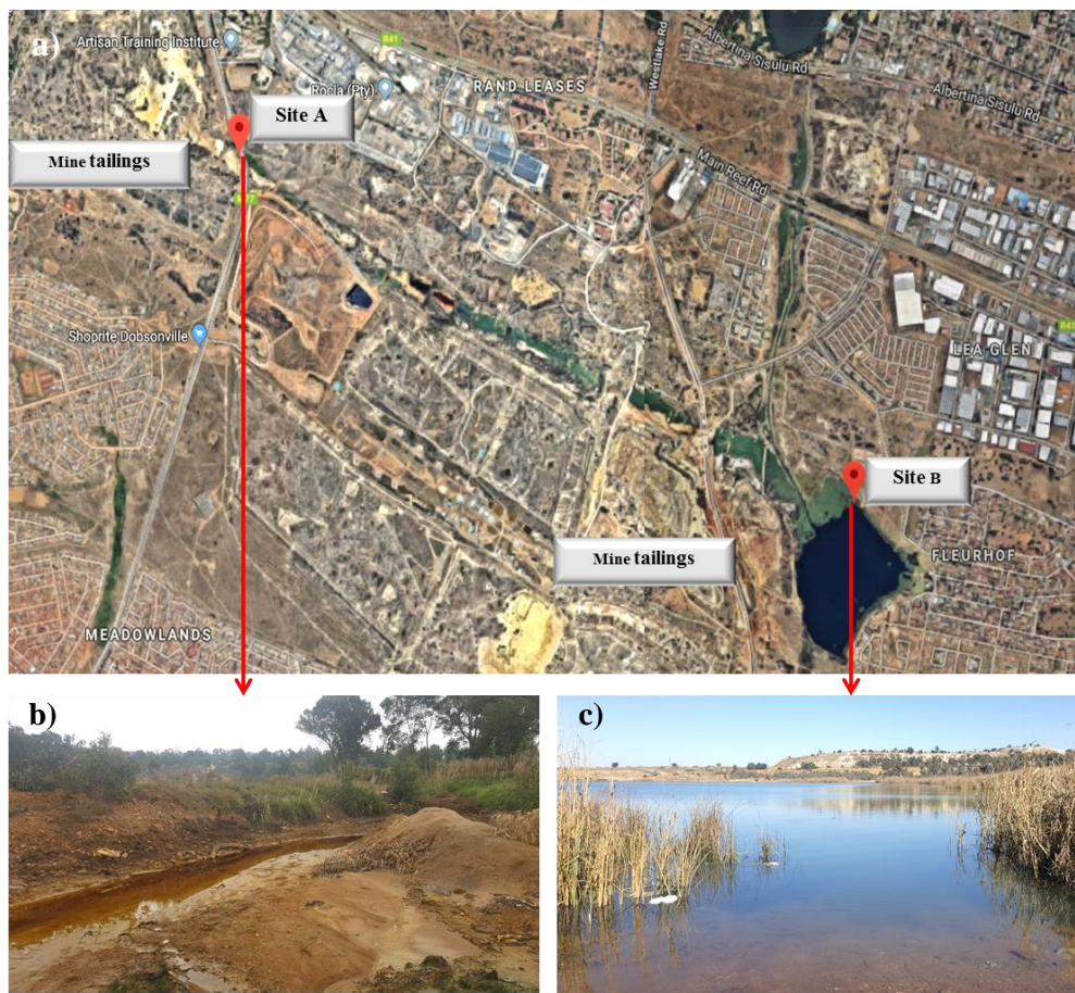
Figure 4.6: a) Aerial view of the area where water samples and DGT passive samplers were deployed: b) site A is the site with active AMD seepage and c) site B is Fleurhof Dam, which is in close proximity to mine tailings and active AMD.
