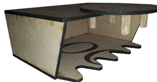
Fig 9.15- Same height joint Where two pieces of a model meet and there is no contour overlap, a building could act as a pin between the two contours as shown in prototype C
