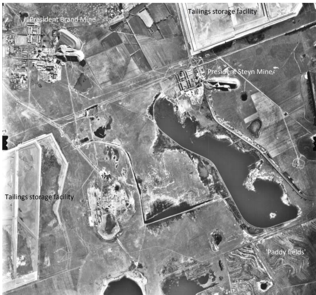
Figure 32. The extensive water management and tailings storage facilities at President Brand and President Steyn mines in 1968 (aerial photo 606_012_00387)
