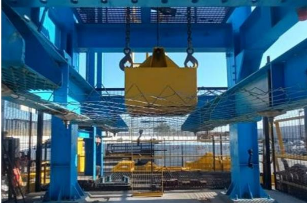
Appendix A-1: Drop test set-up for MINAX 80/3 BOM with spike plates only
