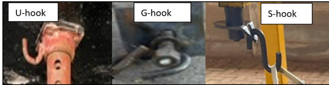
Figure 2-8: Typical safety net hooks used in the South African underground mines
