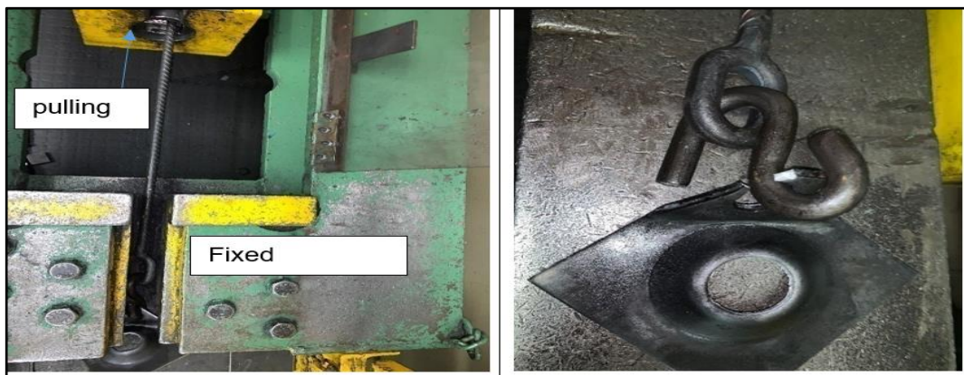
Figure 4-4: Pull test of face plates and hooks (le Roux, 2020)
