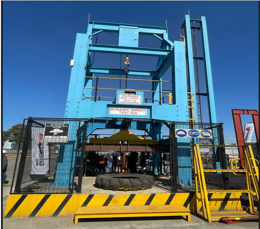
Figure 3-7: Videx dynamic impact drop test facility
