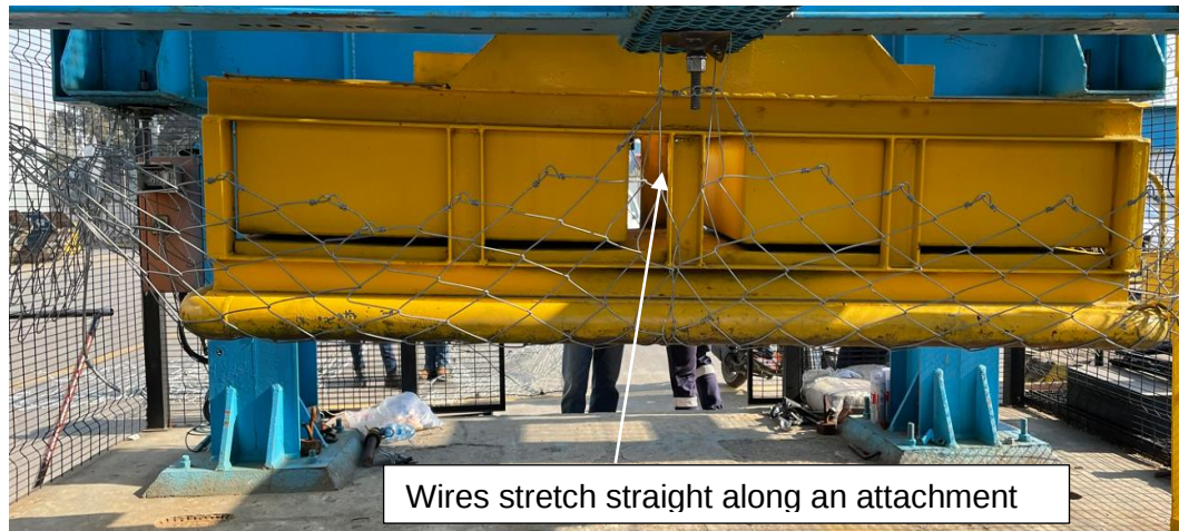
Figure 5-14: Deformation of MINAX 80/3 BOM with face plates at 0 m drop height
