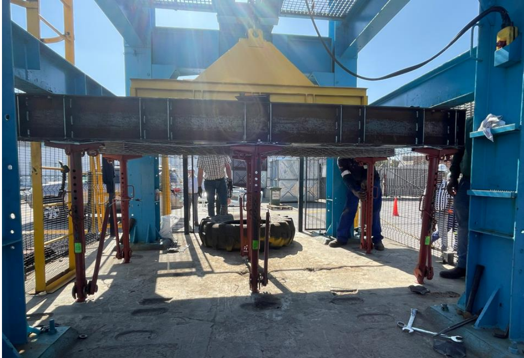
Appendix A-3: Drop test set for MINAX 80/3 BOM with long headboard Videx mechanical props
