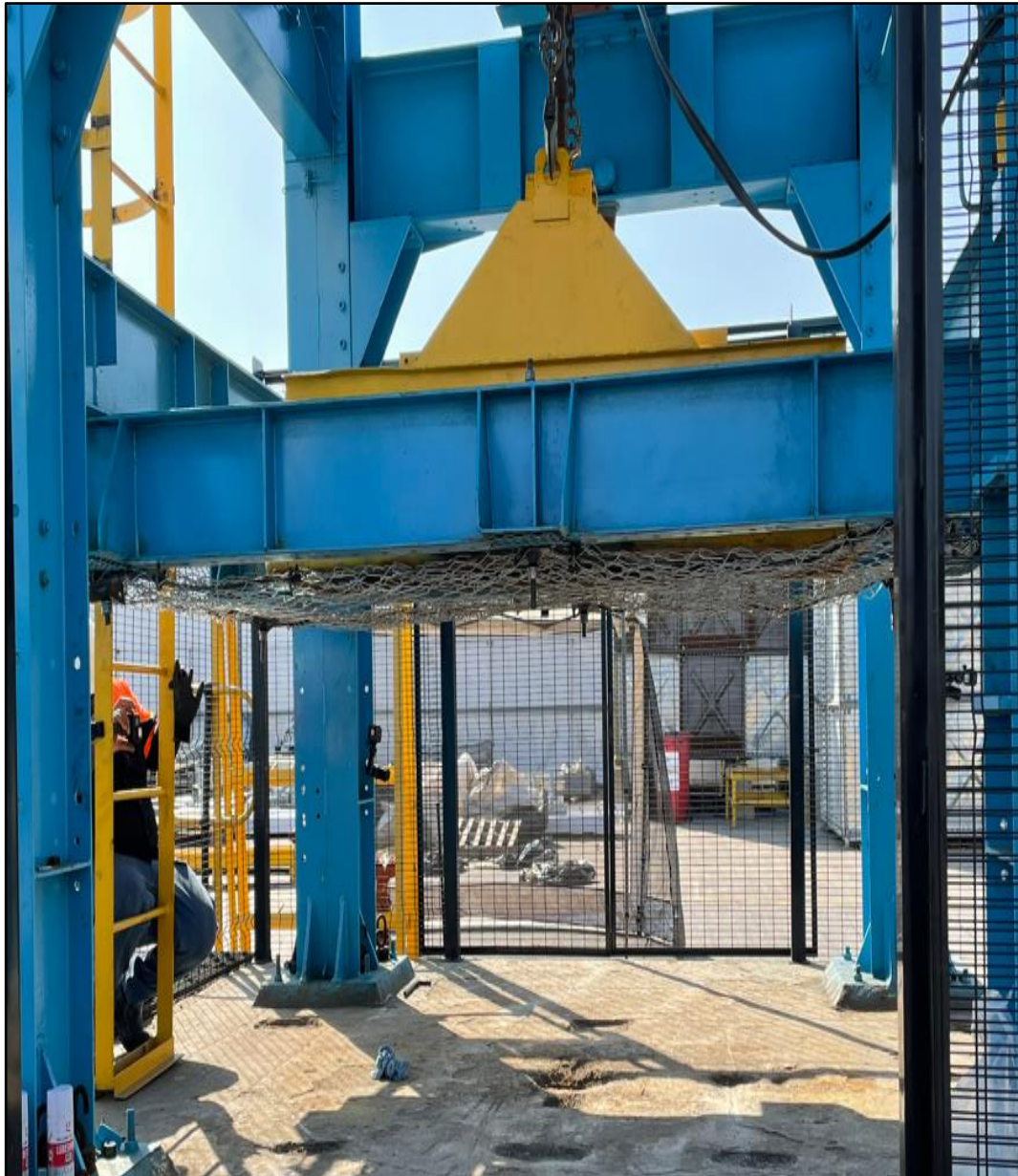
Figure 3-8: Videx drop test base frame
