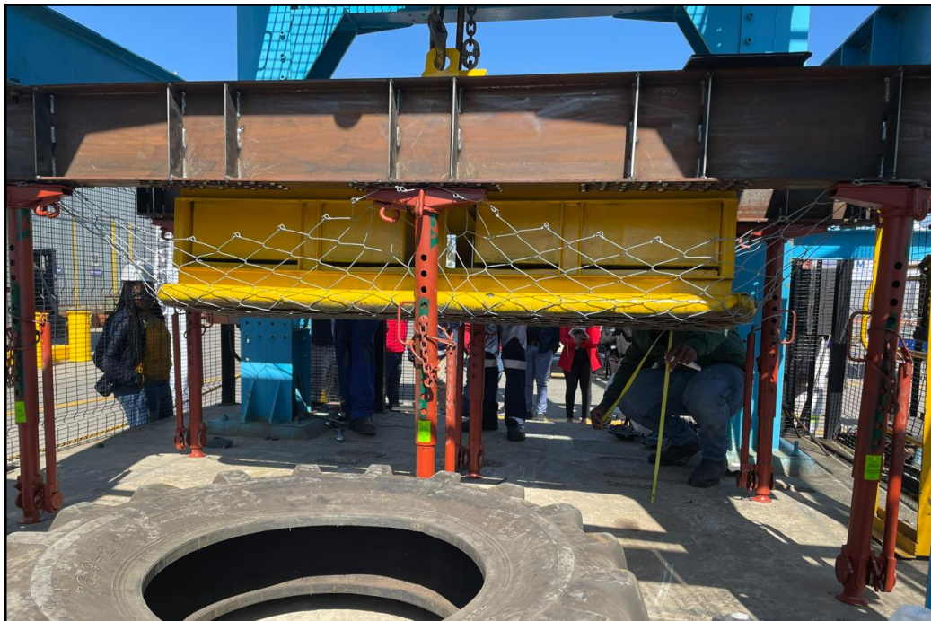
Figure 5-19: Deformation of MINAX 80/3 BOM with mechanical props
