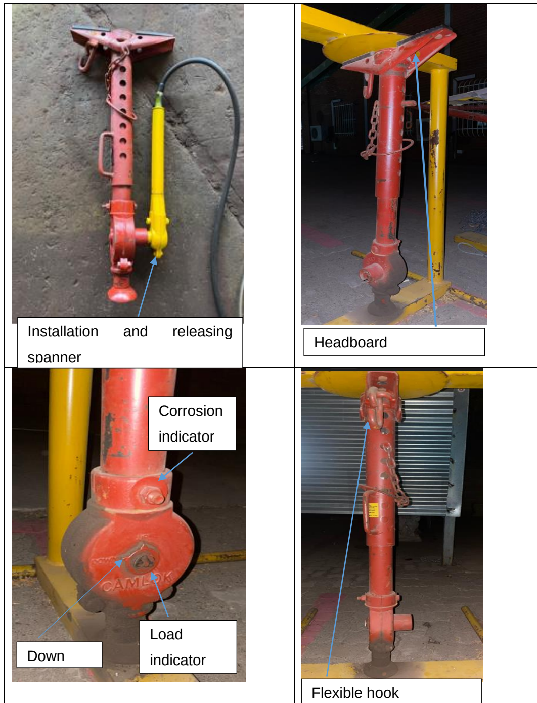
Figure 4-2: T-shaped long headboard Grease box mechanical prop used at Thembelani Mine
