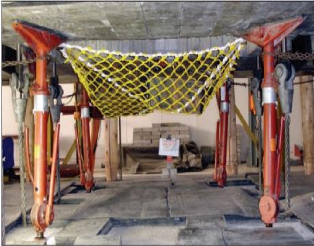
Figure 2-17: Savuka drop test facility set-up simulating gravity-induced FOGs (dynamic testing) (Skarbøvig et al., 2011).
