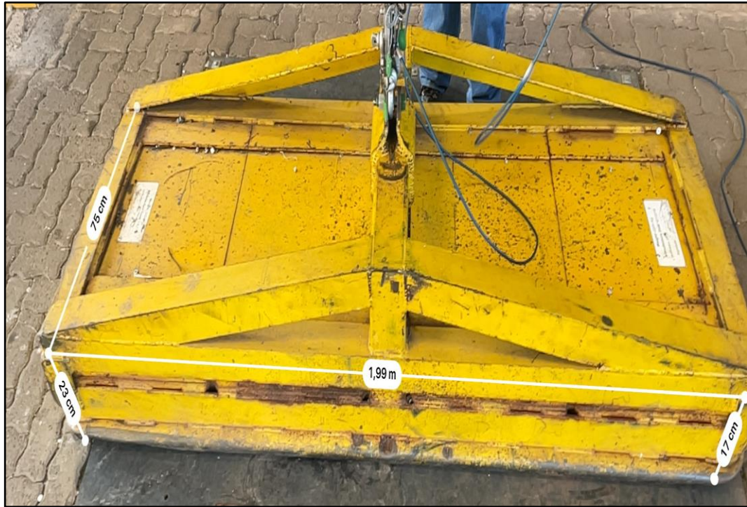
Figure 3-6: Two tonnes steel slab at NCM drop test facility
