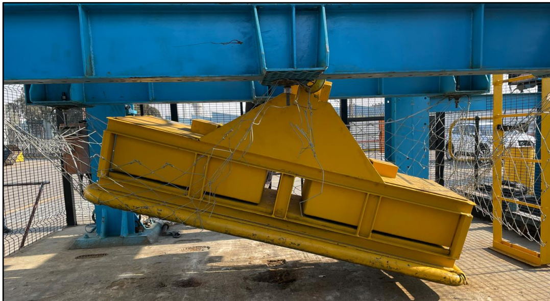
Figure 5-13: Deformation and failure mechanism of MINAX 80/3 BOM with face plates for 0.1 m drop height
