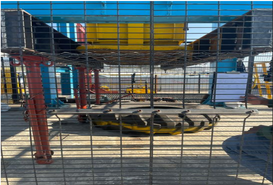
Appendix A-2: Drop test set-up for MINAX 80/3 BOM with mechanical props and spike plates
