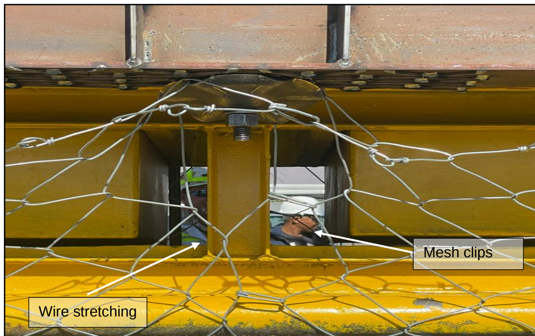
Figure 5-16: Deformation of MINAX 80/3 BOM with spike plates for 0 m drop height
