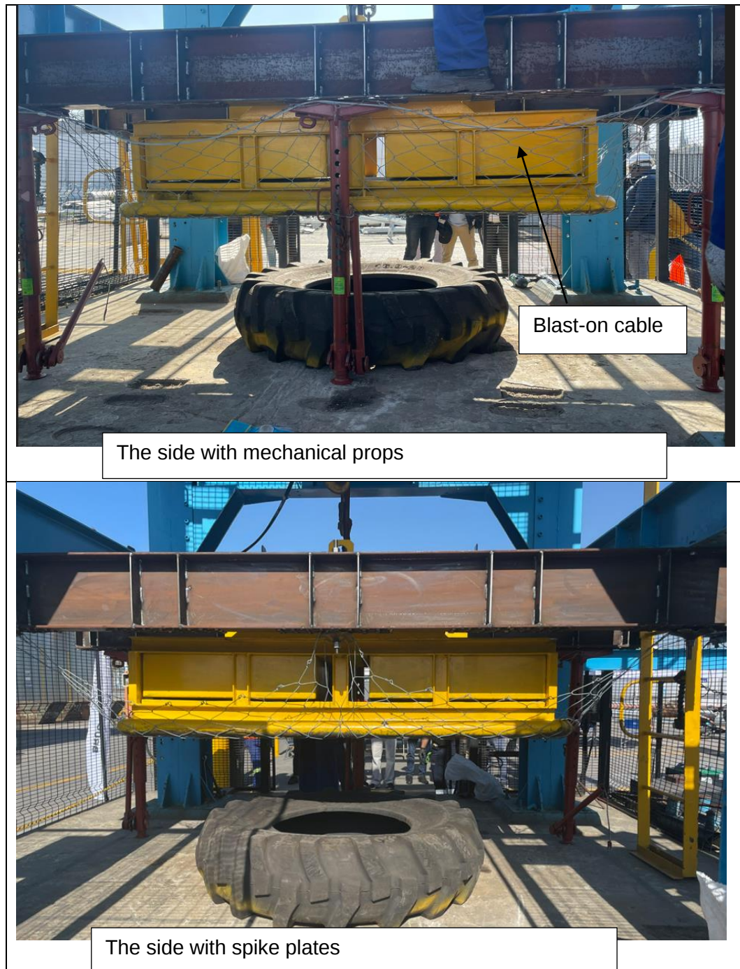
Figure 5-18: Deformation of MINAX 80/3 BOM with mechanical props and spike plates
