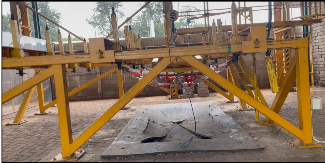
Figure 3-3: NCM Frame 1 for testing of nets, hooks and face plates
