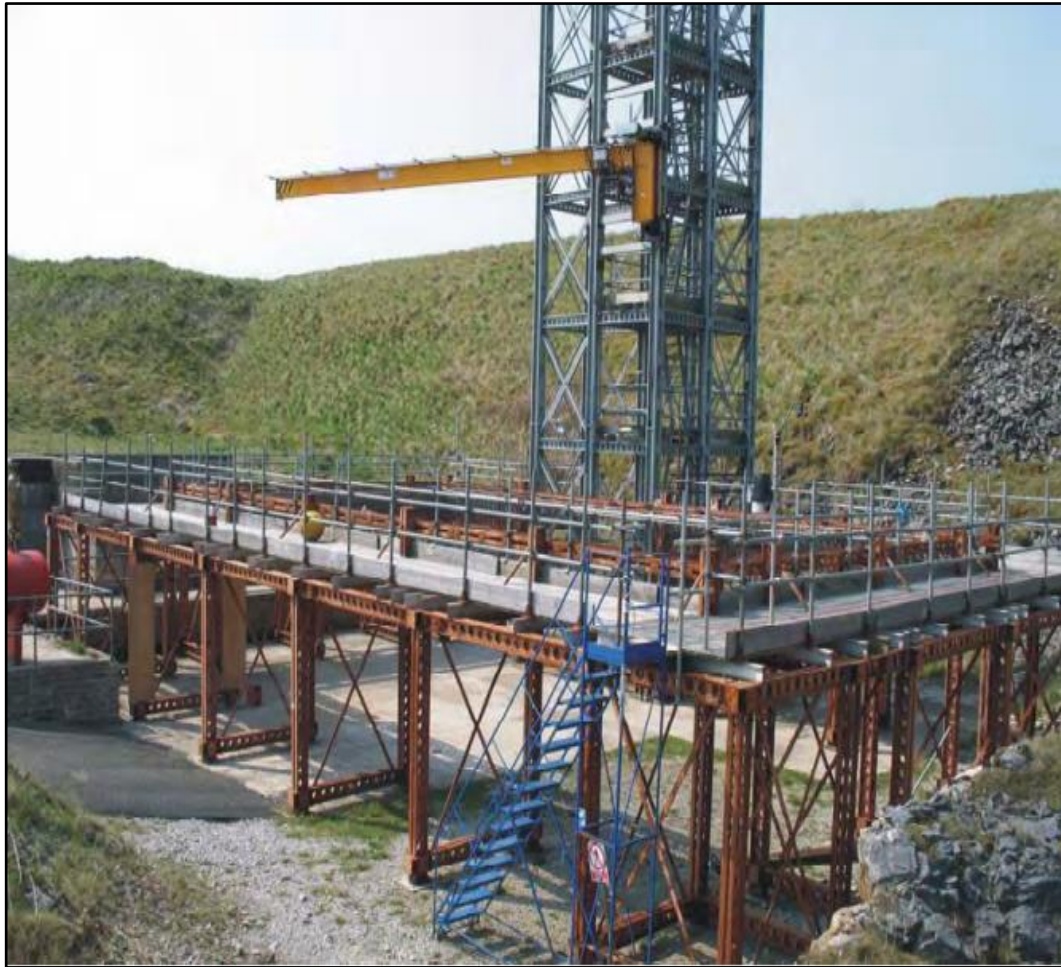
Figure 2-13: Dynamic drop test facility for construction industry safety nets situated in the United Kingdom (McCann, 2011)
