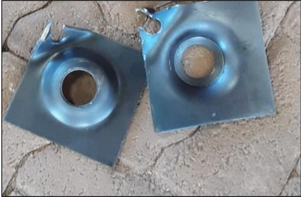
Figure 5-9: Typical failure of the 4.5 mm thick face plates
