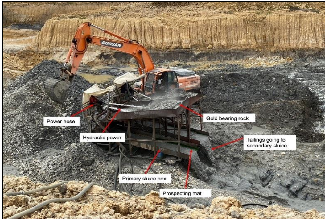
Figure 5.17: Hydraulic mining as conducted by the legal miners
