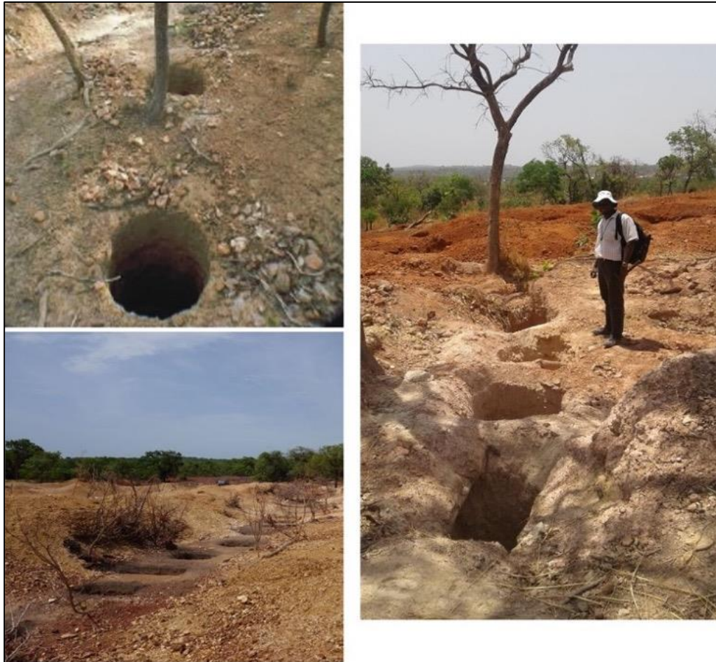
Figure 4.4: Pitting Exploration method. Source: Volcanic Goldmines Inc. (2017); Unity Global Mines Group Inc. (2019).
