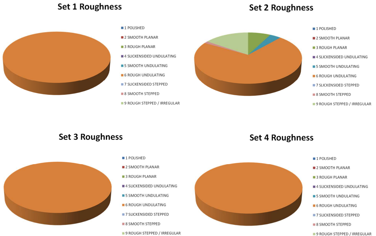
Figure 3-13: Joint roughness for each joint set (Southern Sector)
