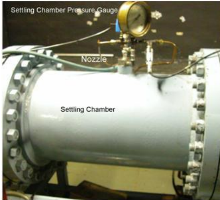
Figure A. 6: Settling chamber.
