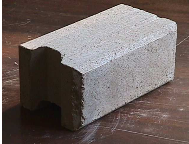
Figure - 2.3: Full scale partition dry-stack block unit
