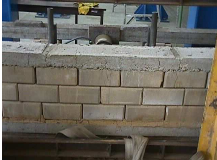
Figure - 5.12: No lateral instability on symmetric section
