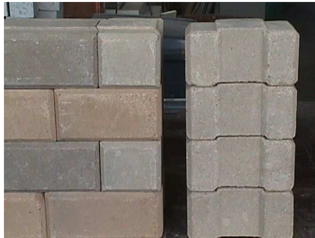
Figure - 3.1: Hydraform blocks stacked to form a wall
