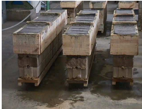
Figure - 5.4: Dry-stack reinforced beams
