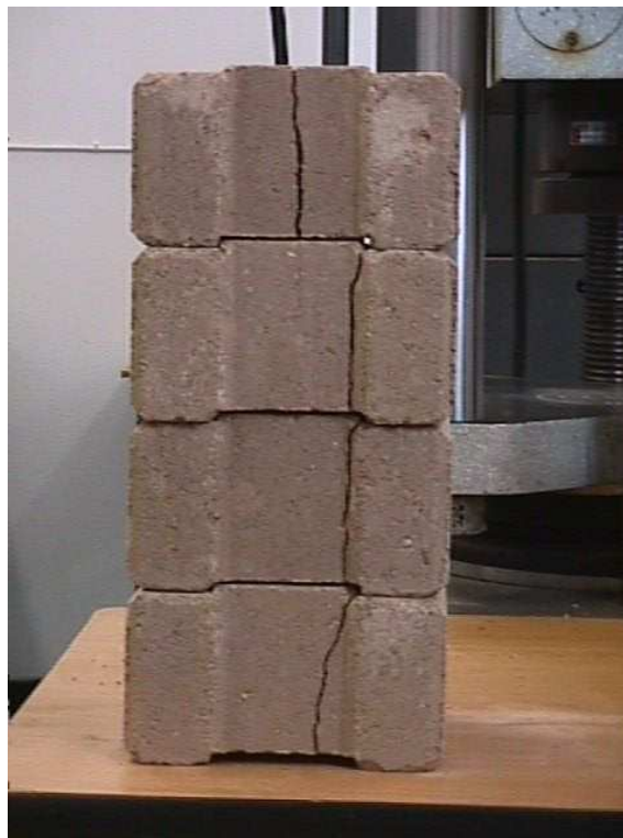
Figure - 4.6: Prism failure mode when loaded at centre
