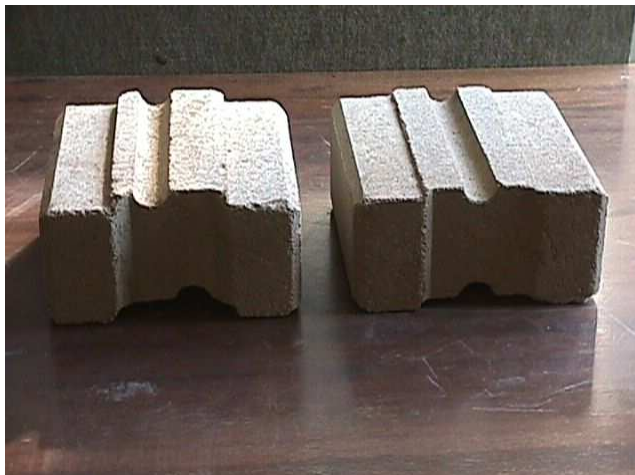
Figure - 2.4: Full scale conduit block units
