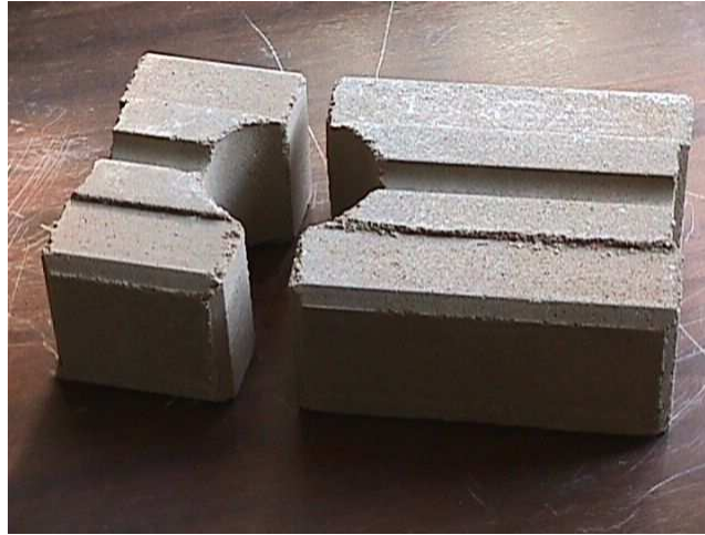
Figure - 2.5: Full scale and corner conduit and grout block units
