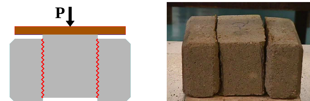
Figure - 3.10: Block unit failure mechanism on centre testing
