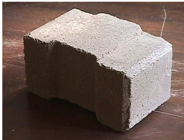
Figure - 2.2: Corner dry-stack block unit
