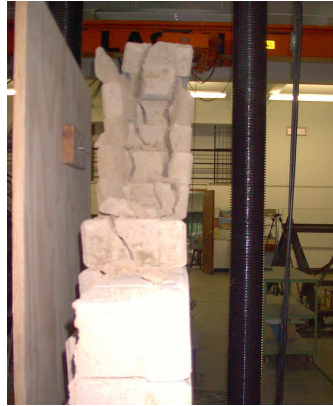
Figure - 4.4: Failure mode of panel made of low strength units (source: Ngowi - 2005)
