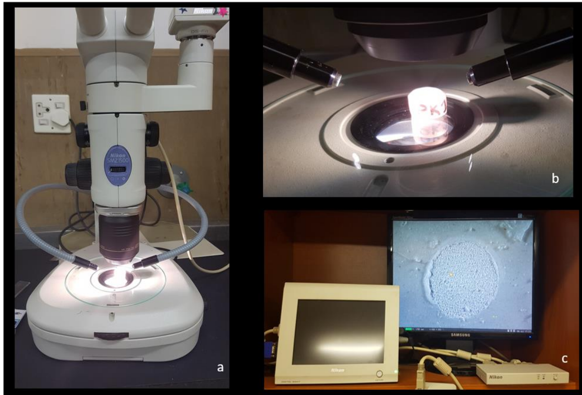
Figure 6: a) Stereo Microscope (Nikon SMZ 1500, Johannesburg, South Africa). b) Failure mode being inspected on a PEEK specimen. View of specimen at 16X magnification projected on monitor
