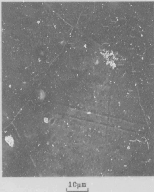
Figure 4.29 Twin impinging on grain boundary precipitates. The round inclusion is a REM oxide. (Alloy V4/0,10, embrittled.)
