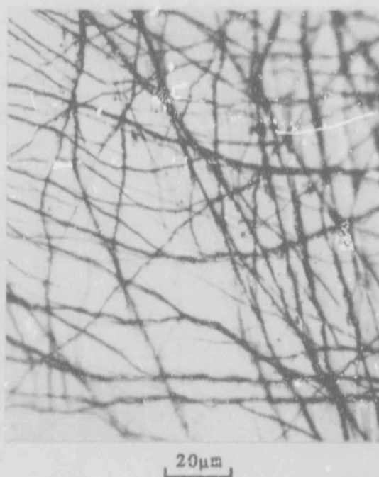
Figure 4.23 Extensive cross-slip associated with ductile fracture. V3/2 tested at 10°C.
