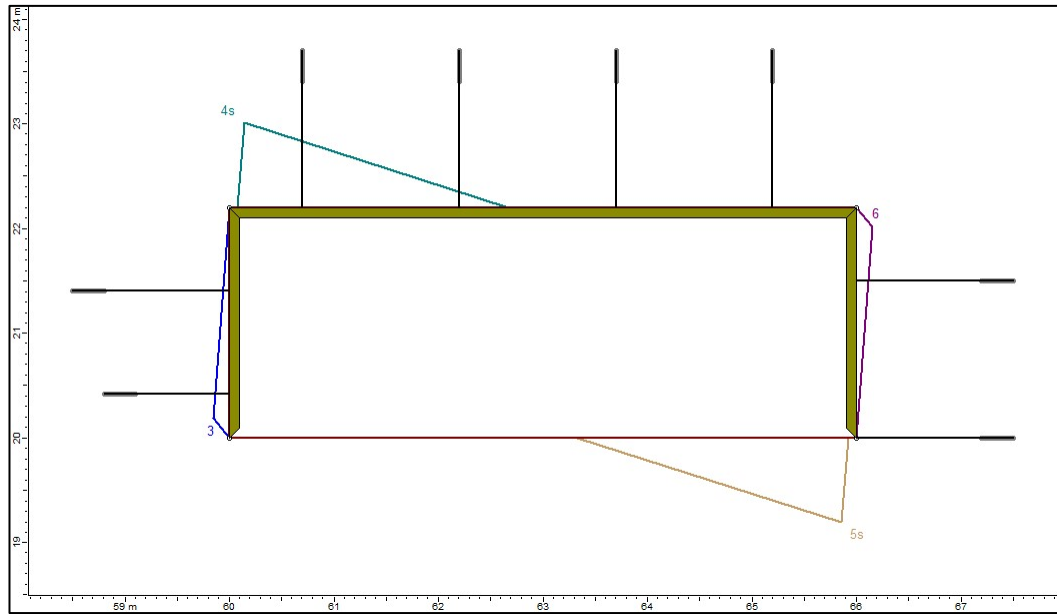
Figure 6-8: 30 mm Shotcrete and 1.5m long resin grouted bolts installed on a 1.5 m by 1.5 m grid spacing in RIG 50
