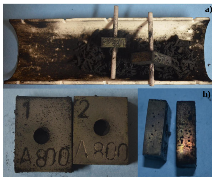
Figure 81. Photographs of the samples after 336 h exposure at 650°C, showing coking (a) and discolouration and pitting (b).
