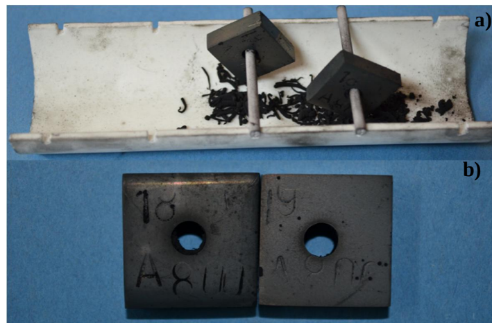
Figure 53. Photographs of the samples after 168 h exposure at a temperature of 650°C, (a) coking and (b) after coke removal (b)..
