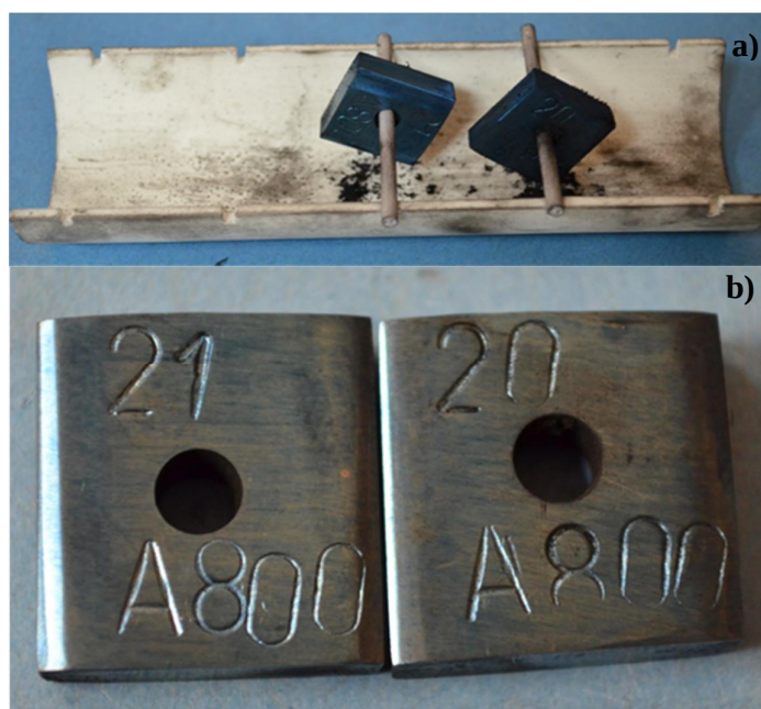
Figure 23. The samples after 72 h exposure at a temperature of 525°C, a) from the furnace and b) removed from the boat.
