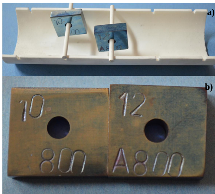
Figure 9. Photographs of the samples after 24 h exposure at a temperature of 525°C, a) from the furnace and b) removed from the boat.
