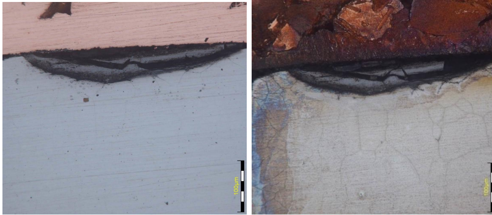
Figure 86. Micrographs of the samples after 336 h exposure at 525°C in the as-polished condition (left) and etched (b) showing a pit on the surface and some grain boundary attack.
