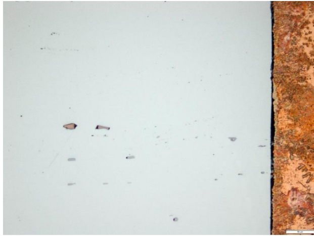
Figure 54. Micrograph of the samples exposed for 168 h at 525°C in the as-polished condition, showing the carbo-nitrite particles.
