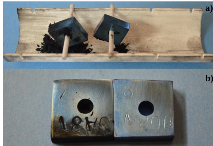
Figure 52. Photographs of the samples after 168 h exposure at a temperature of 525°C, showing coking (a) and after coke removal (b).
