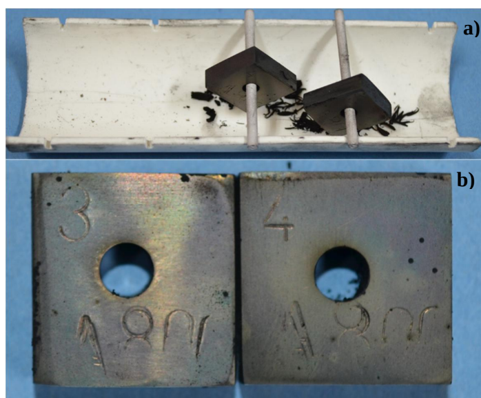
Figure 24. The samples after 72 h exposure at a temperature of 650°C, a) from the furnace and b) removed from the boat.
