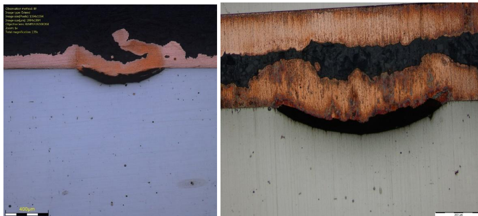
Figure 88. Micrographs of the samples after 336 h exposure at 650°C in the as-polished condition showing pits on the surface.
