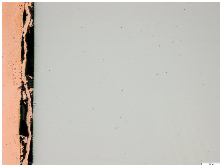
Figure 25. Micrograph of the sample after 72 hr exposure at 525°C.
