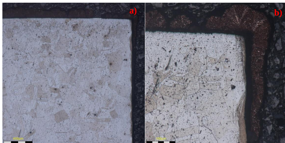
Figure 12. Micrographs of the samples after 24 h exposure at 525°C, after etching, a) low magnification and b) high magnification.
