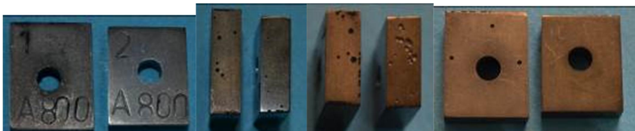
Figure 82. Photographs of the samples after 336 h exposure at a temperature of 650°C, after cleaning, showing discolouration and pitting.
