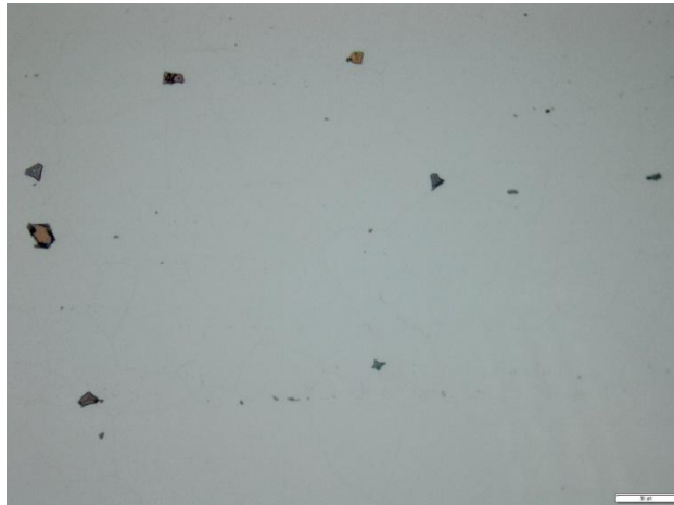
Figure 55. Micrograph of the samples exposed for 168 h at 650°C in the as-polished condition, showing the carbo-nitrite particles.
