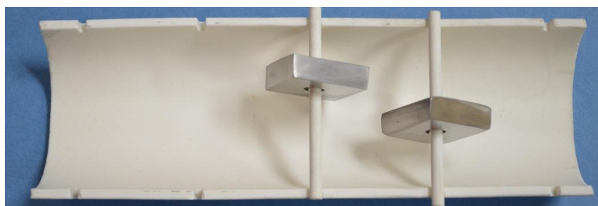
Figure 7. A photograph of the samples illustrating how they were suspended inside the ceramic boat.
