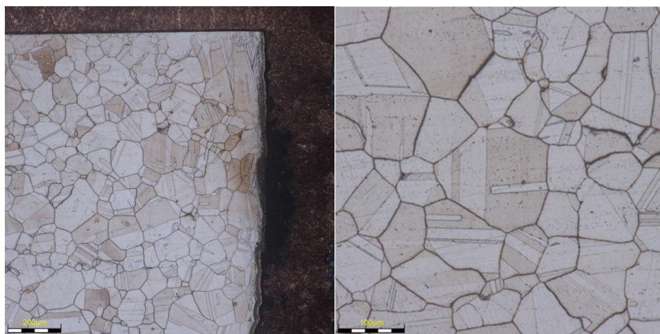
Figure 57. Micrographs of the samples exposed for 168 h at 650°C in the etched condition, showing the carbo-nitrite particles along the grain boundaries.
