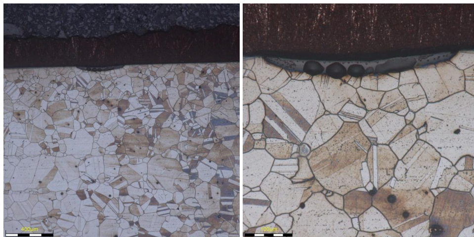
Figure 28. Micrograph of the sample after 72 h exposure at 650°C, after etching showing attack on the edges in a form of a pit, (a) low magnification and (b) high magnification.
