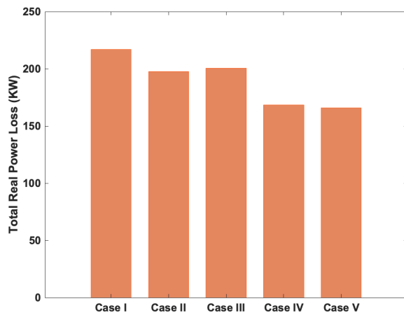
FIGURE 6.5: Total real power loss in a 33-bus distribution network for all cases.
