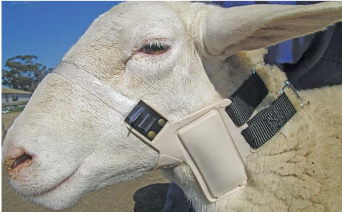
Figure 5.5: Sheep collar device with poisonous pouch
