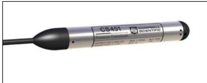
Figure 5-10 Water level sensor (Campbell Scientific, 2017c)
