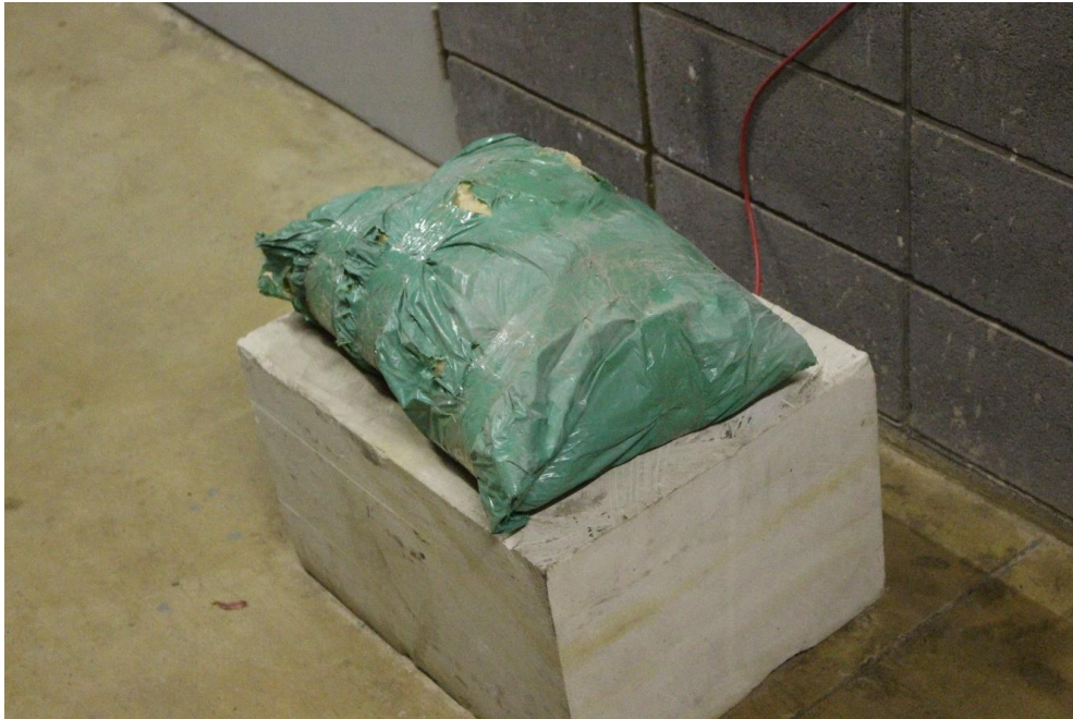
Figure 5-13 Loaded concrete block with stress meter installed inside the block
