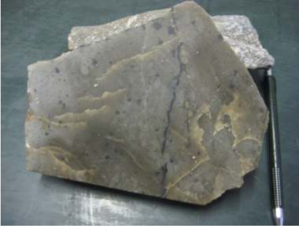
Figure 2.11: A sample of the quartz porphyry dyke from Fairview Mine, which was dated by de Ronde et al. (1991) at 3126 \pm 18 Ma.
