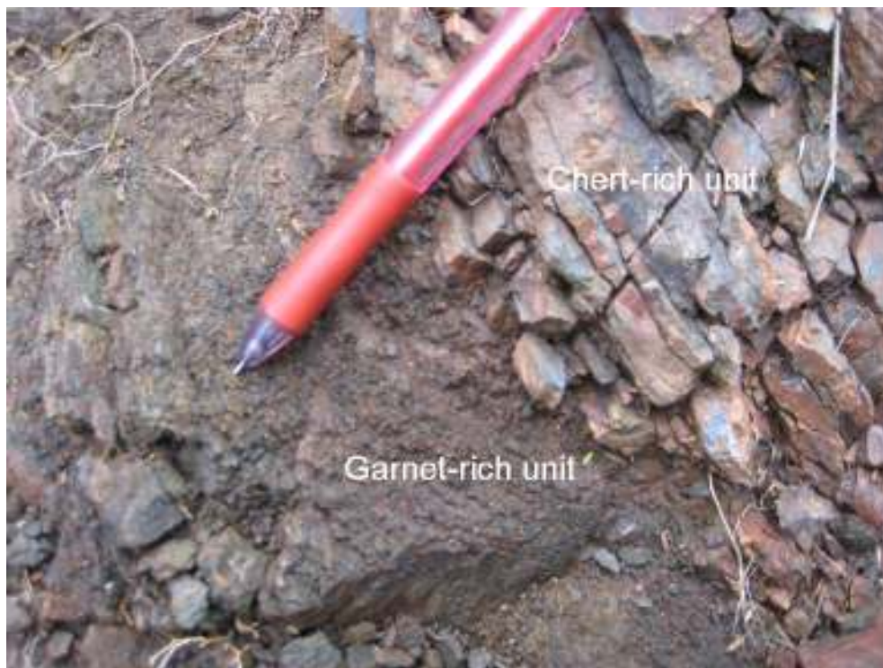
Figure 3.7: Garnet bearing greywacke unit interbedded with chert-rich units (GR 307523-7161049).
