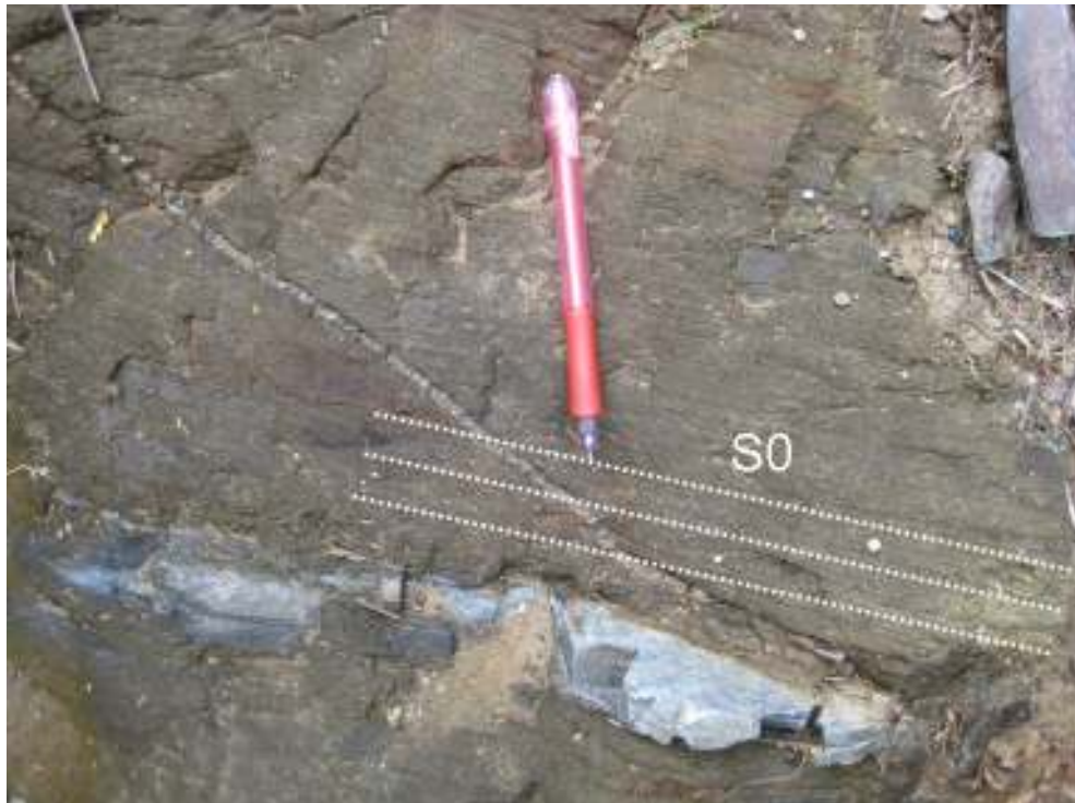
Figure 3.5: Greywacke showing bedding plane (S0) crosscut by chert-rich veins (GR 307513-7161014).
