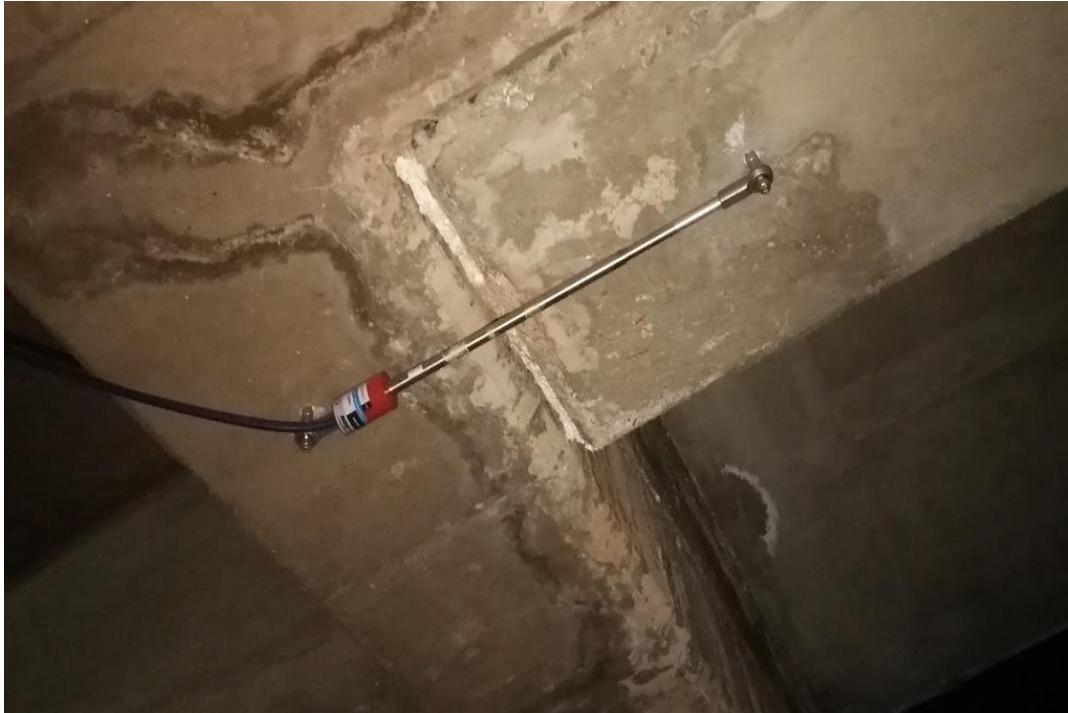
Figure 12: Strain gauge installed on the ceiling in mock mine.
