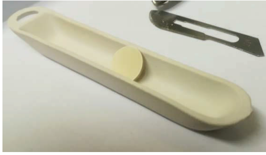
Figure 3.6 A ZnO pellet just after compaction (green body).
