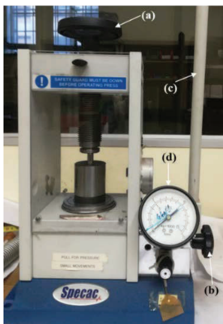
Figure 3.5 The Specac Manual Hydraulic Press, with the pellet moulding die in place. (a) the leadscrew, (b) the pressure release valve, (c) pump handle and (d) pressure/load gauge.
