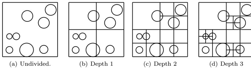
Figure C.2: Building a quadtree. Adapted from [4]
