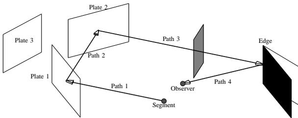
Fig. 2. Ray from a segment to an observer.
