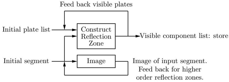
Figure B.5: Block Diagram of the recursive loop for building reflection zones.
