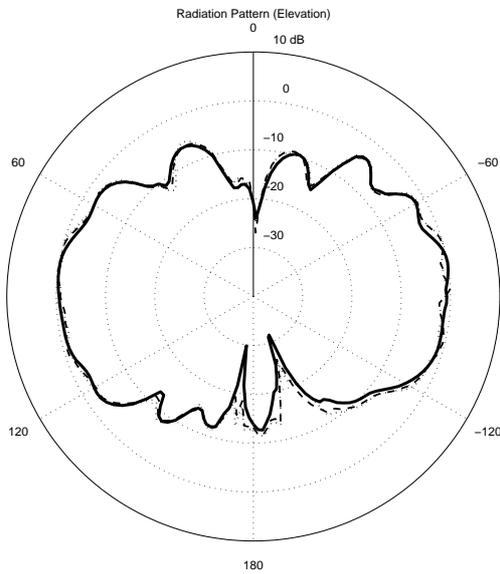
Fig. 14. Radiation pattern ( $\phi = 0^\circ$ ,  $\theta = 0^\circ..360^\circ$ ) for a dipole in the presence of 2 six sided boxes and 2 single plates.
