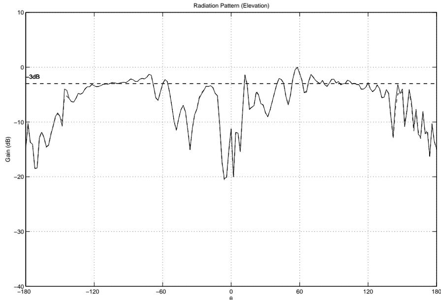
Figure B.16: Radiation pattern ( $\theta = -180^\circ..180^\circ, \phi = 90^\circ$ ) for model 1 using all optimisations.  $m_{ae}=9.04 \times 10^{-2}$  dB
