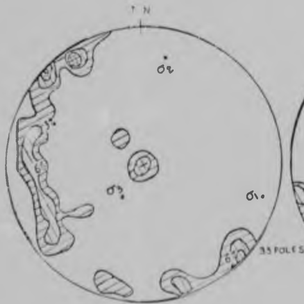
Fig 5,4 Stereograms showing relationship of principal stresses to joint orientation (left) and slickensiding directions on joints (right) Site 1, 23, x/c Bl. 16 2yb level
