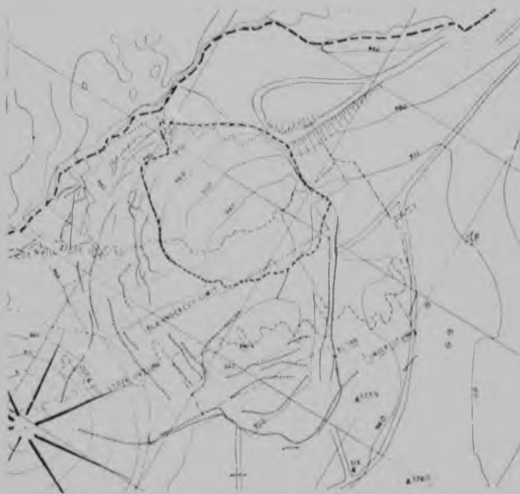
Fig 6.18 Block 7AB surface subsidence zone October 1970 Scale 1 : 2500
