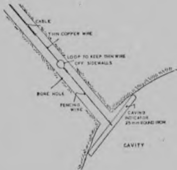
Fig 4,17 Caving Indicator
