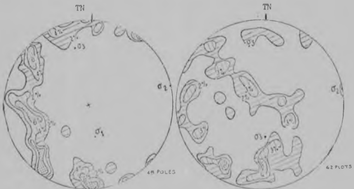
Fig 5.6 Stereograms showing relationship of principal stresses to joint orientation (left) and slickensiding directions on joints (right) Site 3 Main x/c Bl. 33 295 level
