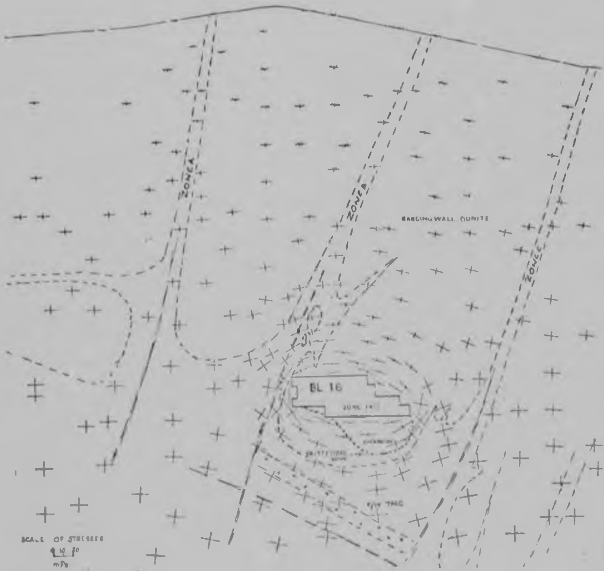
Fig 8.5 Stress directions in and around Block 16 from a finite element analysis
