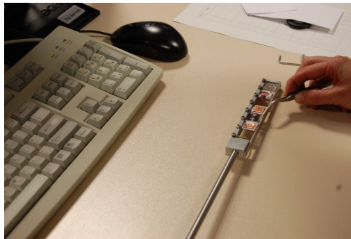
Figure 4.12: Sample holder being attached to the microbeam line sample rod.
