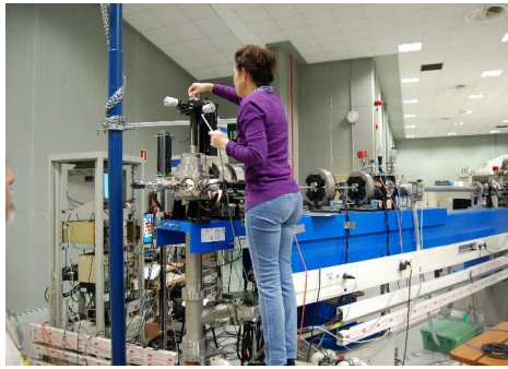
Figure 4.14: Diamond sample being positioned to be in line with the microbeam.
