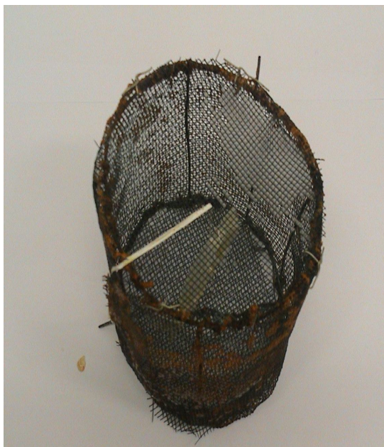
Figure 4.16 Photo of an iron protective cover showing a problem of rusting encountered.
