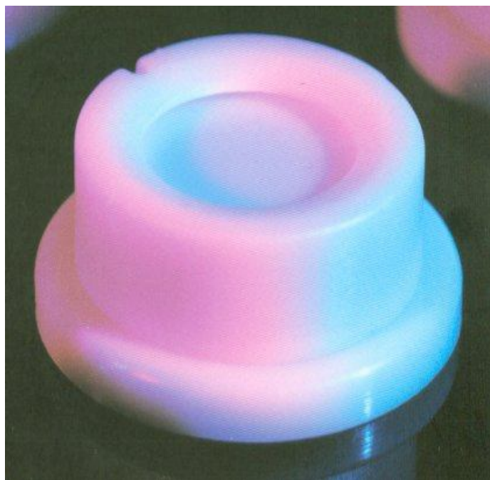
Figure 2.7 Photo (by A. Künzelmann, UFZ) of an exemplary DGT sampler made from plastic as an outer-sleeve placed over the base in order to secure the three layers and maintain an even surface, and to inhibit water ingress into the resin-gel (Zhang and Davison, 1995).
