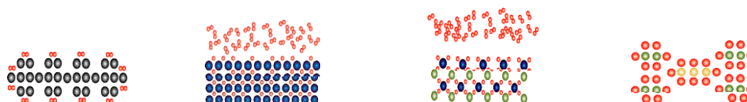
a) Surface adsorption b) Intermetallic hydride c) Complex hydride d) Chemical hydride
