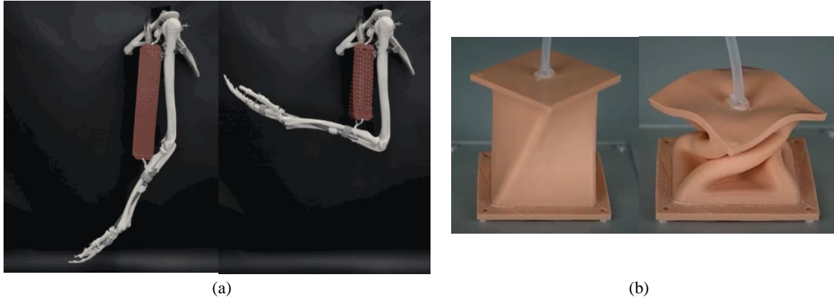
Figure 9: Vacuum-powered soft actuators used for (a) linear [45] and (b) twisting actuation [46].
