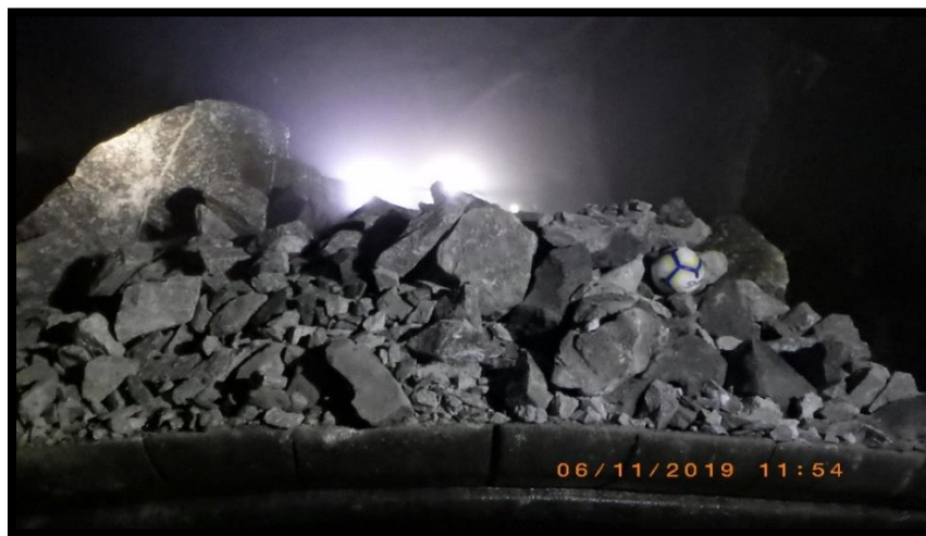
Figure 3.1: Image of an LHD scoop loaded with ore for fragmentation analysis.
