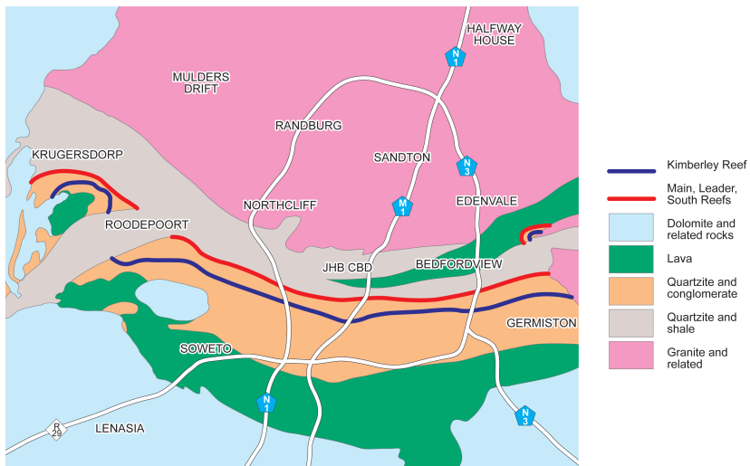
Figure 2: Geological cross-section orientated in a north-south direction showing southerly dip of the layers of sedimentary rock which host the gold-bearing reefs (shown in red and blue). Most of the mining activity was centred along the Main Reef layer with more limited mining of the Kimberley Reef.
