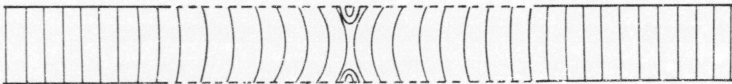
Fig 4.13 a) Lines of constant potential for the boundary conditions given in Fig 4.9
