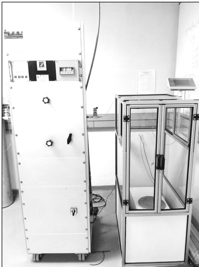
Figure 3.4: Filling station in the gas analysis laboratory used for adding gas into the sample cylinder.
