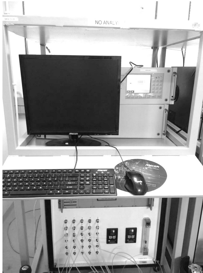
Figure 3.6: Non-dispersive ultraviolet analyser for nitric oxide measurement
