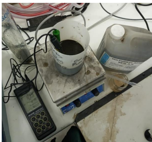
Fig 4.3 Initial pH adjustment using acid/base solution and pH meter for Series 1 experiments
