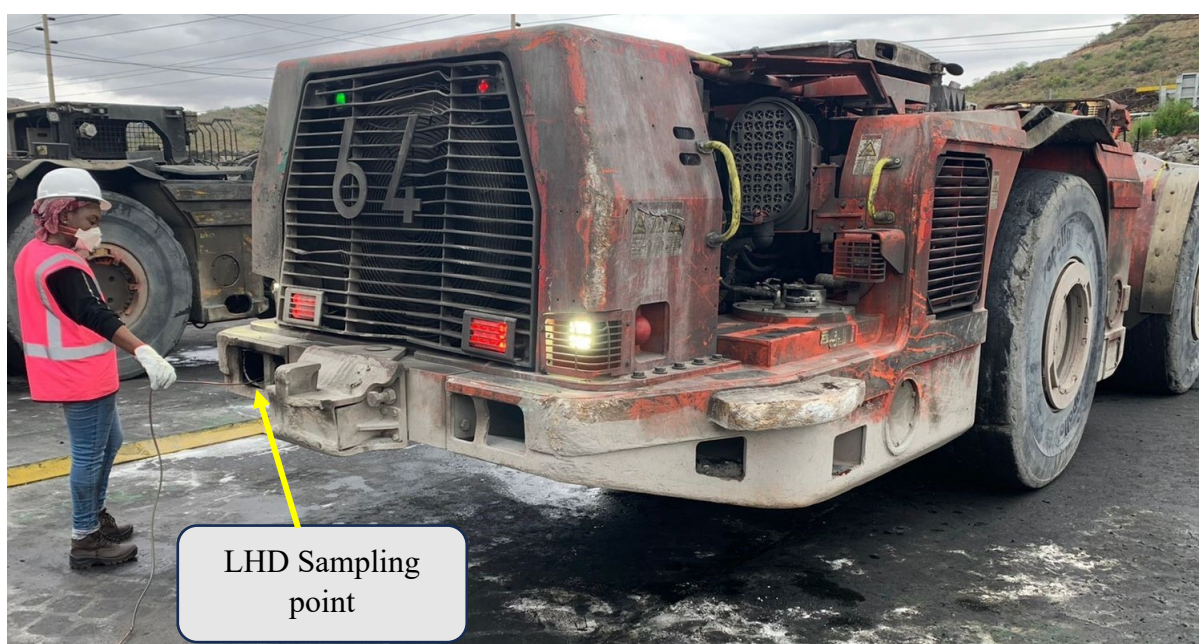
Figure 5.3: Tier II LHD was installed with DPF, showing the sampling point.
