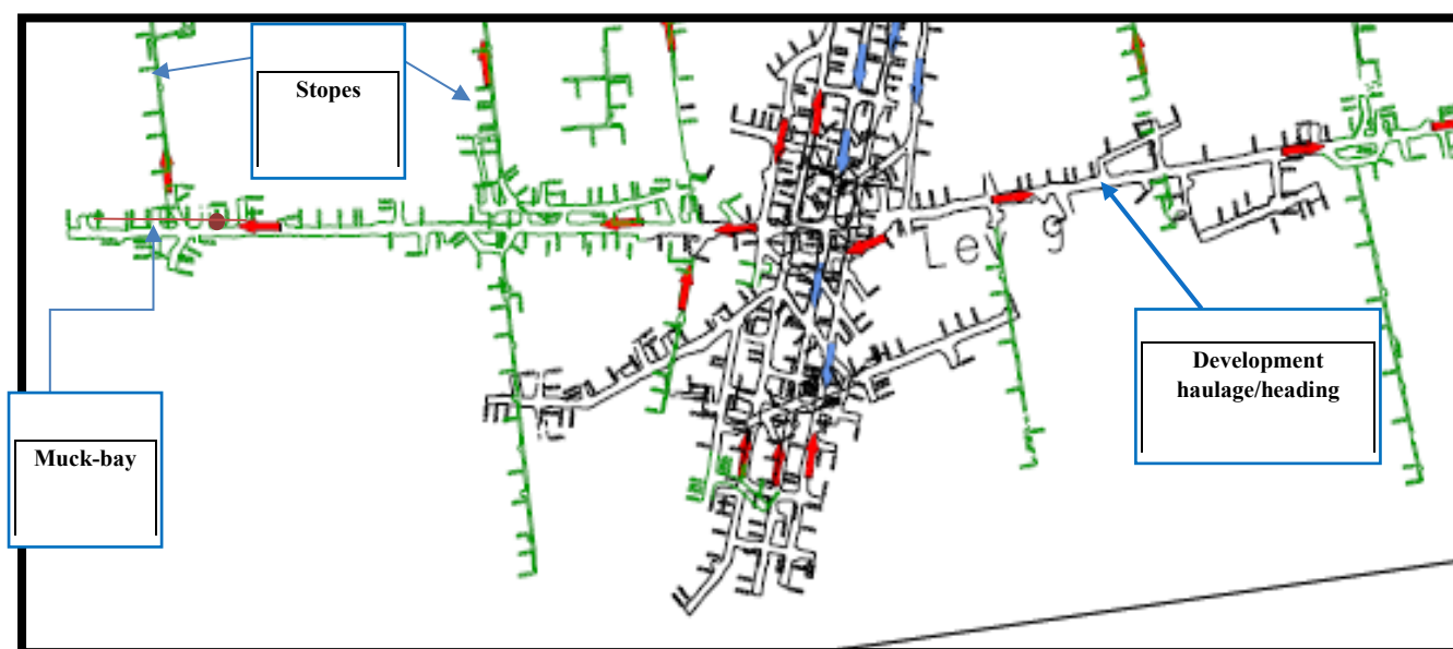
Figure 2.14: This schematic diagram shows a closer view of the Ventilation layout for a flat main development end layout (A—adapted from the CAD plan at Mine at B 2022).
