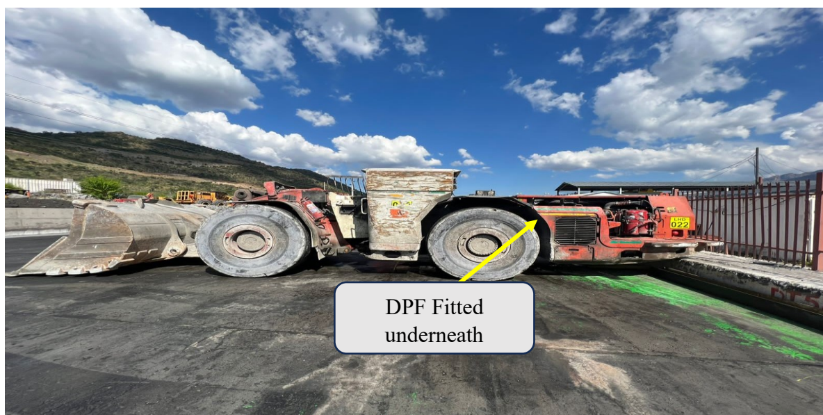
Figure 5.2: Tier II LHD was installed with DPF, as shown in the arrow.
